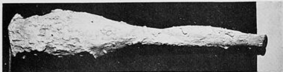
FIG. 1.—Pointed (Service) Bullet, 22 cal.; Cast of Effect in Clay. The tapering of the cast shows the gradual loss of velocity. The bullet is seen at the end of the cast, apex upwards. The narrow part of the cast is where the bullet began to turn over, and the track of destruction changed from cylinder to flat tear.
