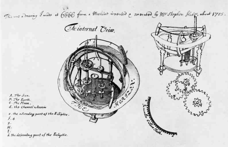
Plate IV. Stukeley's drawing of the machine which Hales constructed to demonstrate the movements of the planets (From the original in the Bodleian Library)
