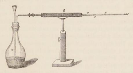
a is the evolution flask, b a tube containing chloride of calcium, c the tube in which, at the point d, the glass splinter with the specimen is placed. This part is then (the apparatus being completely filled with pure hydrogen gas) exposed to a slight heat, at first, in order to expel all moisture, and then suddenly to a very strong heat, (this is best done with a blow-pipe,) to prevent the sublimation of undecomposed sulphuret of arsenic. The metallic mirror is formed near the point e.
