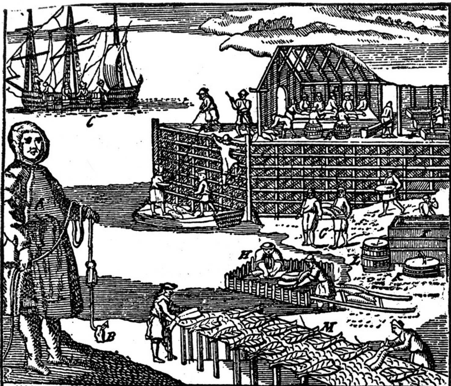
A View of a Stage, also of manner of Fishing for, Curing & Drying of Cod at NEW FOUND LAND :- A. The Habit of the Fishermen. B. The Line. C. The manner of Fishing. D. The Dressers of the Fish. E. The Trough into which they throw the Cod when dressed. F. Salt Boxes. G. The manner of carrying the Cod. H. The Cleansing of the Cod. I. A Press to extract the Oyl from the Cod's Liver. K. A Cask to receive the Water and Blood that comes from the Liver. L. another Cask to receive the Oyl. M. The manner of drying the Cod.
