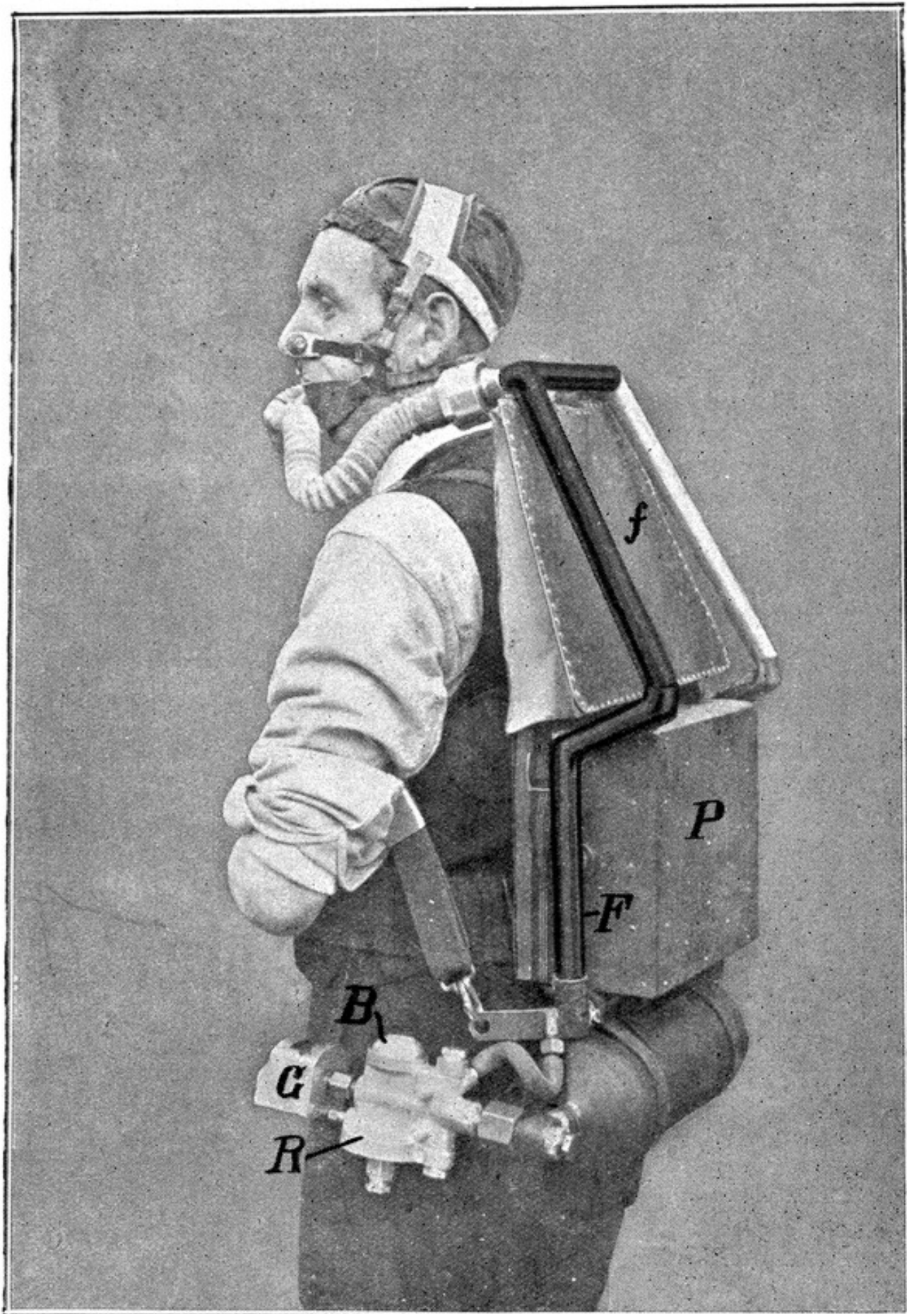
FIG. 87.—The Briggs oxygen-supply apparatus: f , bag; F , cooling tube which also forms frame; P , purifying compartment; B , bye-pass; R , reducing valve; G , gauge. The oxygen cylinder lies below the purifier. The head and mouthpiece is well shown. (From Final Report of Mine Rescue Apparatus Committee, by permission of the Controller, H.M. Stationery Office.)
