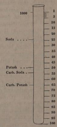
It is convenient, in conducting this process, to set aside a portion of the alkaline liquid, in order to neutralize the acid, in case it should at first be added too freely. To this instrument the term *alkalimeter* is given, a name obviously derived from the use to which it is applied.
