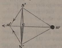
through the centre of motion. This resultant, represented as applied at d, will tend to draw the wire w and the middle of the magnet C directly towards each other. If the conducting wire w were on the right instead of the left side of the magnet, as in figure 16, then
