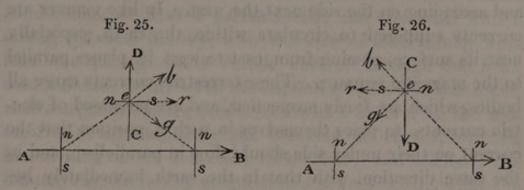
Figure 26 shows the effect of reversing the current in CD, which will consequently be drawn by a force at right angles to itself on the side of A.
