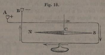
ence of each side, agreeably to the principle above illustrated, will impel the north pole eastward and the south to the west. The little cups A B are designed to contain mercury, and afford a ready means of connecting the rectangle with the opposite sides of a galvanic combination.
