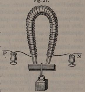
been successfully adopted. The total length of copper wire intended to be used is cut into several portions, each of which, covered with silk or cotton thread to prevent lateral communication, is coiled separately on the iron. The ends of all the wires are then collected into two separate parcels, and are made to communicate with the same Voltaic battery, taking care that the current shall pass along each wire in the same direction. The current is thus divided into a number
