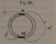
the moment the wires *a b* touched the ends of a Voltaic combination, the galvanometer was strongly affected: the needle then returned to its former position and remained there until the Voltaic circuit was broken, when the needle was again deflected as strongly as before, but in the
