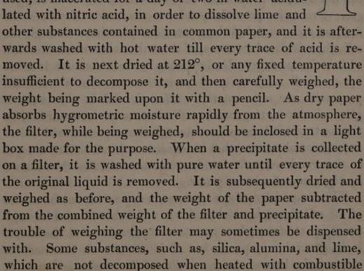
matter, may be put into a crucible while yet contained in the filter, the paper being set on fire before it is placed in the furnace. In these instances, the ash from the paper, the average weight of which is determined by previous experiments, must be subtracted from the weight of the heated mass.
