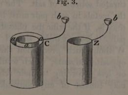
with mercury, and inserting the ends of a wire, the galvanic circuit may be completed or broken with ease and expedition. This apparatus is very serviceable in experiments on electro-magnetism.
