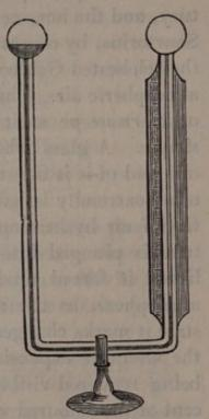
stantly be detected; for the elasticity of the air on one side being then greater than that on the other, the liquid will retreat towards the ball whose temperature is lowest.
