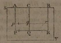
PA, RB, at right angles to AB; and in AP, or AP produced, take PA: pA:: sin. refraction: sin. incidence; and p is the image of P (Art. 120). Draw pr parallel to AB, or PR, and let it meet BR, or BR produced in r; then, since the figures AR, Ar, are parallelograms, RB = PA, and rB = pA; therefore RB: rB:: PA: pA: sin. refraction: sin. incidence;
