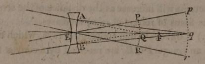
concave lens concentric with PQR, the second image pqr will be erect, or inverted, with respect to the first, according as Q is nearer to, or farther from, the lens than F, the principal focus of rays incident in the contrary direction.
