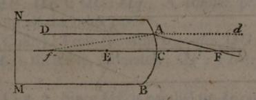
CE :: n : m-n (Art. 131); also, fE : CE :: n : m-n; therefore FC : CE :: fE : CE; or FC = fE. By adding EC to, or subtracting it from each of these equal quantities, FE = fC.
