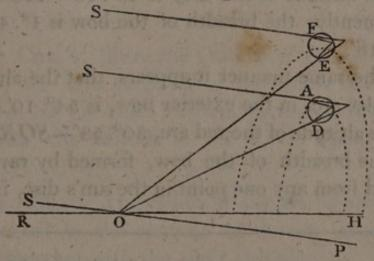
Then the angle ROS, or HOP, measures the altitude of the point S above the horizon; and the altitude
