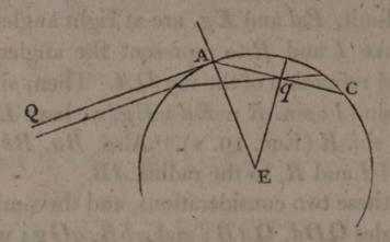
qG vanishes; or q bisects the chord of the arc, cut off by the refracted ray.
