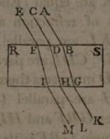
ments of the angles of refraction, that is, the angles SBG, SDH are equal; and therefore BG and DH are parallel.
