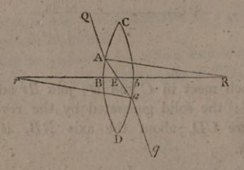
of the lens, in the directions aq, AQ (Art. 29), which are on opposite sides of Aa produced (Art. 33), and in the plane which passes through RA, ra (Art. 24).
