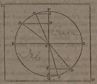
draw the diameters RS, PQ at right angles to each other, and immerse the board into a vessel of water, in such a manner that PQ may be perpendicular to, and RS coincide with the surface of the water. Then, if a ray of light, admitted through a small hole into a dark chamber, be incident upon the surface RS in the direction AC, coincident with the plane of the board, CB, the direction of the refracted ray, is found to coin-
