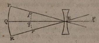
the same way from F, Q and q are on the same side of E; that is, the image is erect. Also, since QF is greater than FE, the object is greater than the image.
