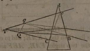
produced, take TC:QC:m:n; then will T be the focus after refraction at the surface IC (Art. 120), or the focus of rays incident upon the surface IB. From T, draw Tc perpendicular to IB, and in cT, or cT produced, take qc:Tc::n:m; and q will be the focus of emergent rays (Art. 120).
