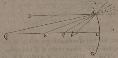
of the pencil, of which QC passes through the center E, and is therefore reflected in the direction CQ; join EA; and, in the plane QACE, make the angle EAq equal to the angle EAQ; then the ray QA will be reflected in the direction Aq.
