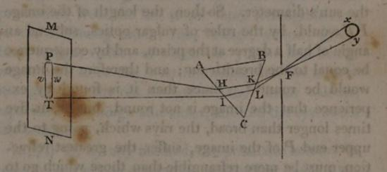
triangular imaginary plane, whereby the prism is feigned to be cut transversely through the middle of the light; and let xy be the sun, MN the paper upon which the solar image or spectrum is cast, and PT the image itself; whose sides, towards v and w, are rectilinear and parallel, and ends, toward, P and T, semicircular. yKHP, and xLIT are two rays; the first of which comes from the lower part of the sun to the higher part of the image, and is refracted in the
