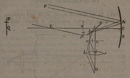
mn in m: take qp equal to nm; draw pE, and produce it till it meets the object in P.
