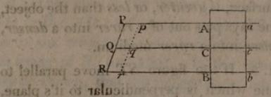
angles to AB; and in AP, or AP produced, according as Ab is denser, or rarer than the surrounding medium, take Pp:Aa:: sin. incidence  $\sim$  sin. refraction: sin. incidence; and p is the image of P (Art. 123). Draw pr parallel to PR, and let it meet BR, or BR pro-
