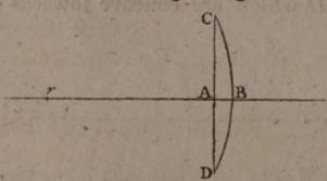
solid generated by the revolution of the figure CD, about the axis rB, is called a plano-convex lens.
