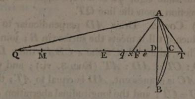
of the pencil to which the ray belongs. Draw AT, touching the arc ACB in A, and let it meet QT in T; bisect ET, EC, in e and F; take q the geometrical focus, conjugate to Q; and let QA be reflected in the direction Ax; also, let Fe be small when compared with QF.
