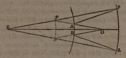
the image seen (Art. 65); join Ep, Er, and let these lines cut the object in P, R, and PR is the corresponding part of the object.
