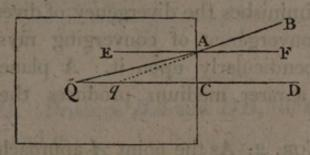
EAQ is equal to the alternate angle AQC, and the  $\angle$  BAF is equal to the interior and opposite angle AqC; therefore, sin. EAQ, or sin. incidence, = sin. AQC = sin. AQq; and sin. BAF, or sin. refraction, = sin. AqC = sin. AqQ; hence, QA: qA:: (sin. AqQ: sin. AQq::) sin. refraction: sin. incidence. Now, let A approximate to C, and QA is ultimately equal to QC,
