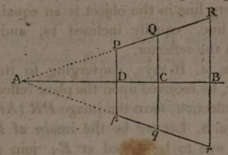
and make Br equal to RB; join Ar; and from P draw PDp perpendicular to AB, meeting Ar in p; then will pr be the image of PR.
