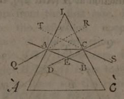
to it's surfaces (Euc. 8. and 18. 11); QA a ray incident in the plane AIC; AC, CS the course of the refracted ray, in that plane (Art. 24). Then, the effect of the refraction is the same, whether we suppose the ray to pass thus through the prism, or AC to pass both ways out of the prism (Art. 30); let this latter supposition be made, and the proposition resolves itself into the three following cases:
