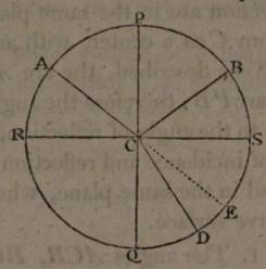
drawn, through C, perpendicular to RS, and AC be produced to E; then ACP is the angle of incidence, PCB the angle of reflection, and BCE the angle of deviation.
