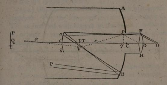
the angles are small, the  $\angle pGq$ : the  $\angle peq$  (TeV):: eq:qG; and also, the  $\angle TeV$ : the  $\angle TEV$ :: ET: eT; by comp. the  $\angle pGq$ : the  $\angle TEV$ ::  $eq \times ET$ :  $qG \times eT$ ; that is, the visual angle, when the object is seen through the telescope: the visual angle, when it is seen with the naked eye::  $eq \times ET$ :  $qG \times eT$ .
