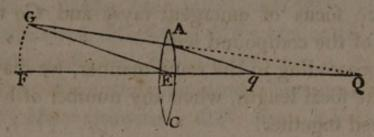
Qq; and q lies between Q and E; consequently, the refracted rays converge more than the incident rays.
