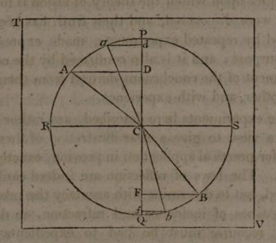
from A, in the direction AC; and since the motion of light, in the same medium, is rectilinear (Art. 10), the ray, by which the object is seen, is incident at C, and refracted in the direction CA.
