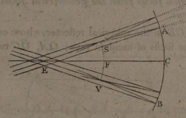
reflector, the foci of reflected rays will lie in the spherical surface SFV, whose center is E and radius EF.
