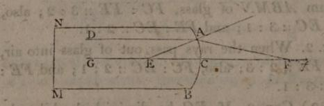
$Ef: EC:: n: m \sim n$ ; also, EF: AF:: n: m; therefore  $EF: EF \sim AF:: n: m \sim n$ ; hence  $Ef: EC:: EF: EF \sim AF$ ; but  $EF \sim AF$  is less than EA, or EC (Euc. 20. 1); consequently, EF is less than Ef.
