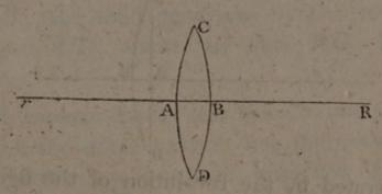
and which meet in C and D; join Rr, and suppose the figure CD to revolve about Rr as an axis; the solid, thus generated, is called a double convex lens.
