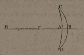
and which meet in C and D; join Rr and produce it to B; the solid generated by the revolution of the figure CD, about the axis RB, is called a meniscus.
