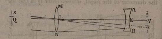
object in S. Then, all the rays which flow from S, or from any point between S and Q, and fall upon the object glass, will be refracted to the eye\*; and QS will be the linear magnitude of half the bright part of the field of view. Also, QS is measured by the angle SLQ, which is equal to sLq = BLE - BLs = BLE - LBN + LsN; and 2 QS is measured by 2 BLE - 2LBN + 2LsN.
