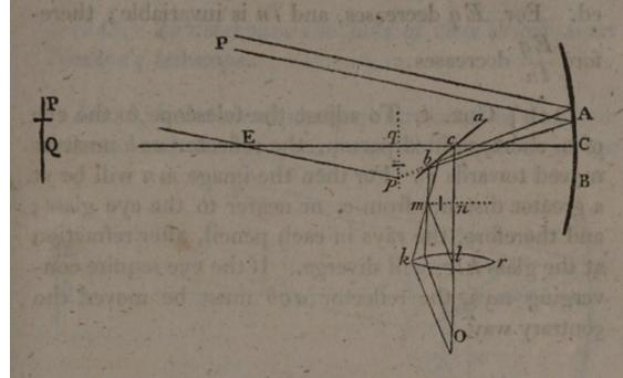
seen through the glass klr, under an angle which is equal to mln; and QP is seen, with the naked eye placed at E, under an angle which is equal to qEp; and since these angles have equal subtenses nm, and qp, they are to each other inversely as the radii ln, qE; therefore the angle which the object subtends at the center of the eye, when viewed with the telescope: the angle which it subtends at the naked eye:: Eq:ln.
