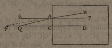
refraction. Through A, draw EAF parallel to QC; and let QA be refracted in the direction AB; produce BA till it meets CQ, or CQ produced, in q\*. Then, the  $\angle EAQ$  is the angle of incidence of the ray QA, and the  $\angle BAF$  the angle of refraction; also, the  $\angle$
