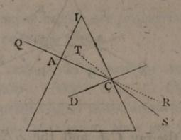
DCI is equal to the sum of the two ACI, AIC, take away the common angle ACI, and the remaining angles DCA, AIC are equal; consequently AIC: ACT::  $m: m \sim n$ .
