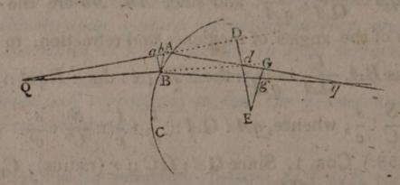
in a plane which passes through it's center E; and let Aq, Bq, be the refracted rays. Draw EdD, EgG, and Ba, Bb, at right angles to QA, qA, or to those
