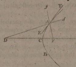
touching the reflector in A; then the angle EAF is equal to the angle DAT, in the ellipse, and to dAT in the hyperbola; therefore AD is the reflected ray in the former case, and Ad in the latter; thus D is the focus of reflected rays.
