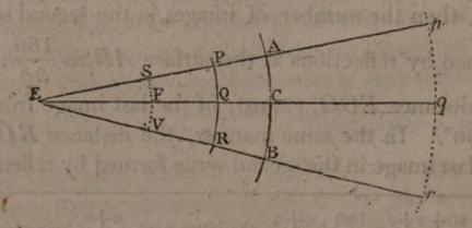
produce these lines, if necessary; bisect EC in F, and take FQ : FE :: FE : Fq, measuring Fq and FQ in the same direction from F; with the center E and radii Eq, EF, describe the circular arcs pqr, SFV,
