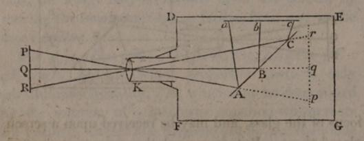
top and the bottom; for the point a, which corresponds to p, or to P in the object, is the farthest point in the image from the reflector; and therefore, the farthest point from the spectator. But, with respect to the right and the left, the image will be inverted. For, the axis of a pencil of rays which flows from a point in the object to the right of Q, will cross the axis Qq at the center of the lens, and the rays will be
