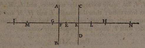
E draw the indefinite right line NEI perpendicular to AB, or CD. Take FG = FE; KH = KG; FI = FH, &c. Also, take KL = KE; FM = FL; KN = KM, &c.
