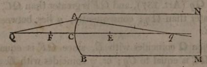
medium diverging from Q, a point farther from the surface than F, they are made to converge.
