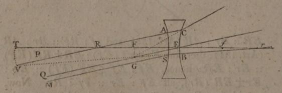
MS a pencil of parallel rays incident upon it; of which QE passes through the center, and may therefore be considered as proceeding in that direction after
