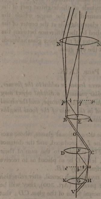
in a; join aG, Ca; and produce Ca till it meets the lens HK in H; draw HV parallel to aG; and at V let the eye be placed. Then, NBCHV being the course of the pencil of rays which flows from P; and LEFGV the course of the pencil which flows from Q,
