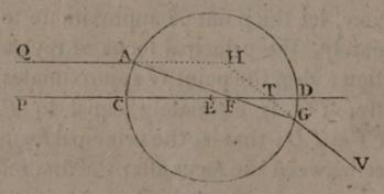
within the sphere; and the rays, after the second refraction, diverge from T.
