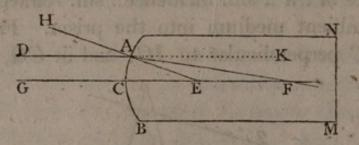
into a denser, the  $\angle EAF$  is less than the  $\angle HAD$ , and therefore it is less than the  $\angle KAE$ ; add to each the  $\angle AEF$ , and the two angles FAE, AEF are together less than the two KAE, AEF; and therefore they are less than two right angles (Euc. 29. 1); consequently, AF, and GE, if produced, will meet.
