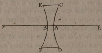
EC, FD parallel to Rr, and equally distant from it; then the solid generated by the revolution of the figure ECDF, about the axis Rr, is called a double concave lens.
