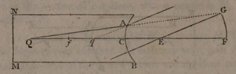
or QA produced, in G; join EG; draw Aq parallel to EG, and let it meet the axis in q.
