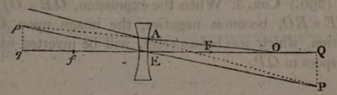
by an eye placed at O. Take qp the image of QP, and join pO. Then, the visual angle pOq varies as  $\frac{qp}{Oq}$ . Now, QF: FE (:: QE: Eq) :: QP: qp; therefore,  $qp = \frac{QP \times FE}{QF}$ . Also, QF: FE:: Ef: fq; whence,  $fq = \frac{FE \times Ef}{QF}$ ; and, when EQ is greater than EF, Oq = fq + Of (Art. 188) =  $\frac{FE \times Ef + QF \times Of}{QF}$  =  $\frac{FE \times Ef + QF \times Of}{QF}$  =  $\frac{QE \times Of - FE \times EO}{QF}$ ; therefore,  $\frac{qp}{Oq}$  =
