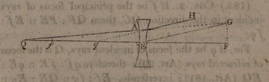
and degree, whether it be considered as belonging to the focus Q, or to the focus G, AH is parallel to GE (Art. 169). Hence, the triangles QGE, QAq are similar, and QG: QE: QA: Qq; therefore, ultimately, QF: QE: QE: Qq.
