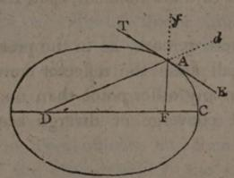
revolution of which, about it's axis, the reflecting surface is formed; F the focus of incident rays; then will D be the focus of reflected rays.
