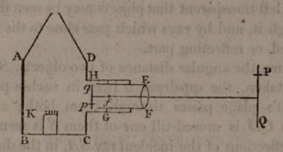
is formed at some distance from the lens (Art. 221), and painted in it's proper colours upon a screen placed at the concourse of the refracted rays.
