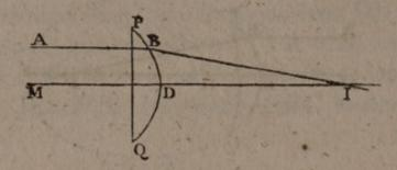
Q, the solid generated by the revolution of PDQ, about the axis MDI, will refract all the rays, incident parallel to MI, accurately to I.
