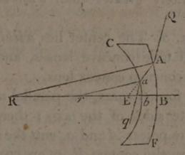
of deviation, are equal; and these are alternate angles; consequently, AQ and aq are parallel.
