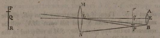
pqr in p; join also, LB, Lp; and suppose pL, EL to be produced till they meet the object in P and Q. Then, QP, which is half the linear magnitude of the
