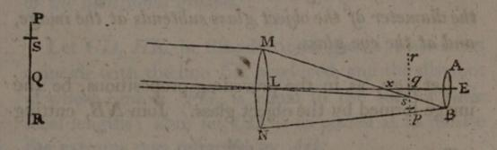
object in S. Then, if xE be greater than qE, all the rays which flow from S, and fall upon MN, will be refracted to the eye glass; for, SM is refracted in the direction MsB; and any other ray of the pencil, as SL, crosses MB at s, and falls somewhere between A
