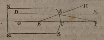
the angle of incidence DAE, or it's equal AEC, is less than the angle of refraction HAF; add to each
