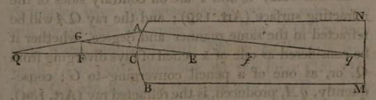
of the pencil, of which QCE passes through the center, and therefore suffers no refraction. Take F the principal focus of rays incident in the contrary direction, parallel to EC; and from the center E,
