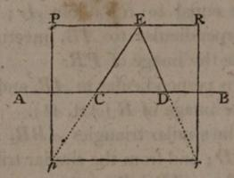
cutting the reflector in C and D; then, considering the pupil as a point, the image will be seen in the part CD of the reflector; and it will subtend the angle CED at the eye; because all the rays enter the eye as if they came from a real object pr (Art. 65).
