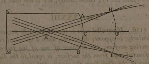
parallel rays be inclined to each other, in the same plane, the foci of refracted rays will lie in the circumference of a circle, HFI, whose center is E, and radius
