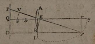
P; join PE, and produce it. Let F be the principal focus of rays incident in the direction qE; with the center E, and radius EF, describe the circular arc FV, cutting PE in V. In PEp, take PV: PE: PE: Pp, measuring PV and Pp in the same direction.
