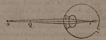
point farther from the eye than Q, will be formed within the eye; therefore, the rays which proceed from this point, will be diffused over some space upon the retina; and, if they are mixed with the rays which diverge from other points in the object, necessary to be distinguished from the former, the vision will be
