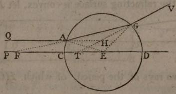
that ray which passes through the center, and therefore suffers no refraction at either surface (Art. 27); also, let QA, any other ray of the pencil, be refracted in the direction AG, and emergent in the direction GT, or GV, which, produced backwards, or forwards, as the case may require, cuts the axis in T. Produce QA, and TG, or VG, till they meet in H; join EA, EG.
