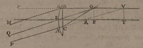
Vr is parallel to ER, and the figure GERV becomes a parallelogram; therefore  $EG = RV = R \times \frac{n}{m-n}$ .
