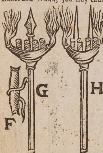
after another, in filling a roll of Canvas sewed together, (as the Figure F sheweth) with flow Receipt, and coated as before is shewed: and this being placed artificially upon the short Barrels or Pipes (as the Figures G H sheweth) and primed with fine Powder directly against the touchholes of the Barrels, pasting a little Paper over the fame, firing the said Trains at both ends, which as they burn, shall still
