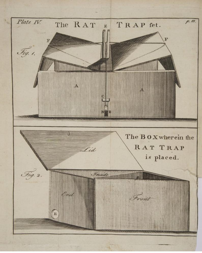
trap, which must be set up about six or seven inches high at each end. The intent of having the under pieces but six inches high, is, that you may be enabled to take them out with the greater safety; for when you place the small wire cage at the end of the trap, then lift the end thereof level or even with the small hole at the side of the cage, and there will be sufficient room for the Rat to go into the cage very easily.
