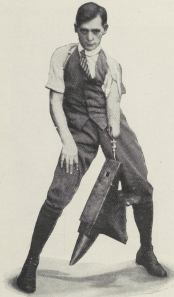
FIG. 119.—BLATCHFORD'S B 1 ARM. The anvil shown weighs 58 pounds. This is a test of the efficiency of the harness.
