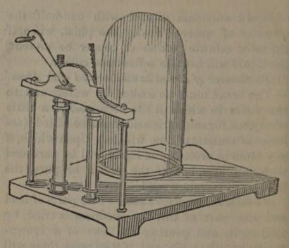
The Air Pump.—The above figure represents the cheapest form, and in action it exactly resembles the common sucking pump, with this difference, that the valves are made of moistened bladder instead of leather
