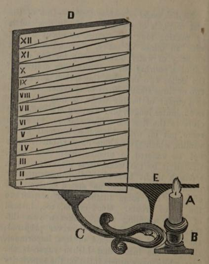
The Lamp Chronometer.—It represents a chamber-lamp, A, consisting of a cylindrical vessel made of tin, in the shape of a candle, and is to be filled with oil. This vessel should be about three inches high, and one inch diameter, placed in a stand B. The whole apparatus of lamp and stand can be purchased, ready made, at any tin shop in London. To the stand B is fixed the handle C, which sup-
