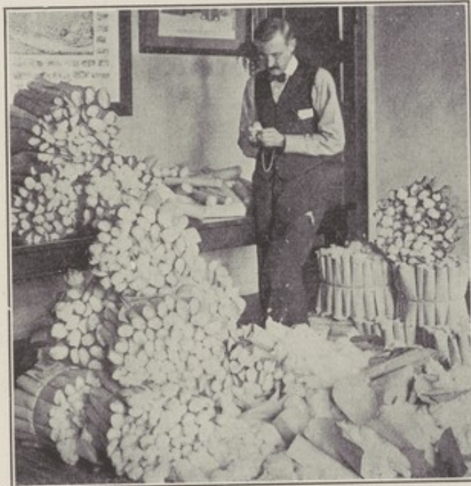
Examining cotton from the bales. Each paper roll contains a sample from a bale.
