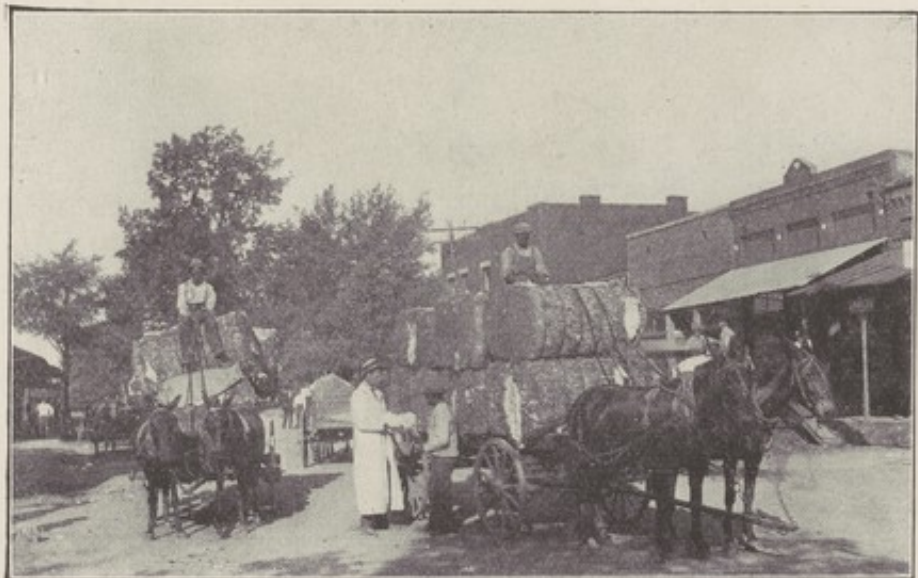
The separated cotton fiber, compressed into bales at the ginning mill, is now on its way to the shipping point.
