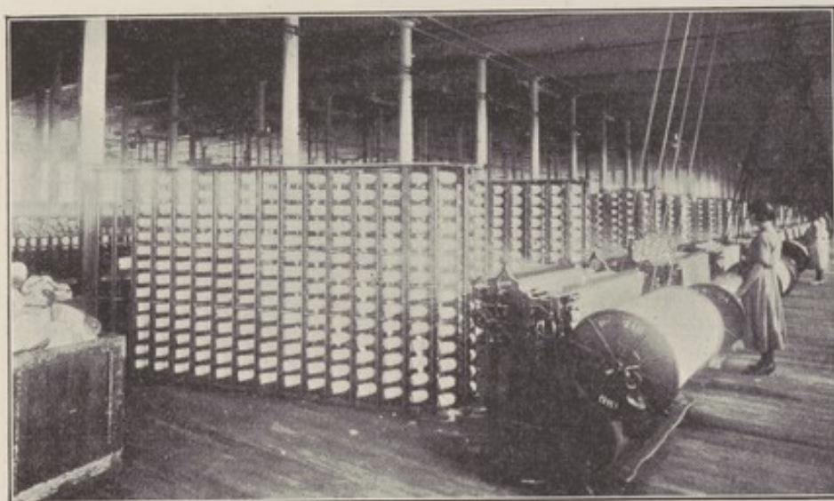
Winding the lengthwise or "warp" yarns on the large drum or cylinder, which later is placed on the weaving loom. As many spools are used on the rack as will supply the desired number of warp yarns required by the yarn. Chicopee Mfg. Co.
