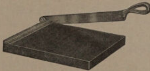
FIG. 1121.—Modified Eastman print trimmer for rough trimming of casts. ( Suggested by Dr. Varney Barnes. )
