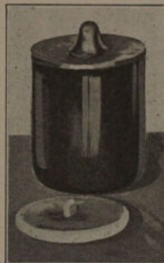
FIG. 470.—Glass tank made from brown bottle. Paraffin float cover and modeling compound tank cover.
