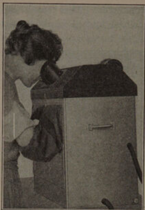
FIG. 400.—Developing the cabinet provides a portable dark-room of great convenience for dentists who wish to do their own work but have no available space for a dark-room.
