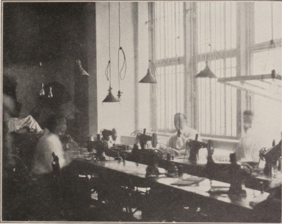
Fig. 1.—Machines, shop No. 18 (on first and second floors), showing poor lighting arrangement. (Note absence of lamps from reflectors.)
