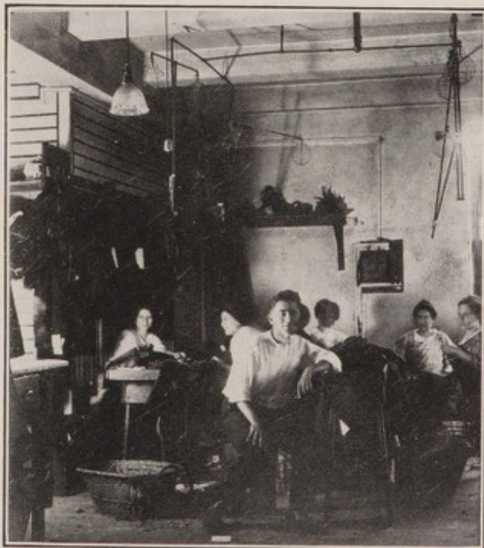
Fig. 6.—Finishing tables, shop No. 10c. Artificial light provided by fishtail gas burners. These let down when in use.
