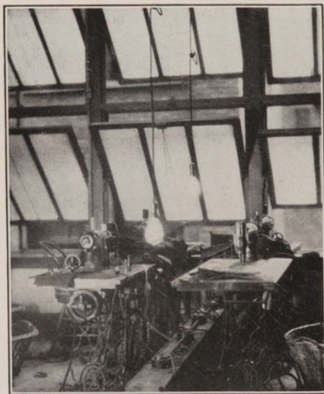
Fig. 4.—Bare lamps used in the illumination of machines. Deep bowl or cone reflectors should be used.
