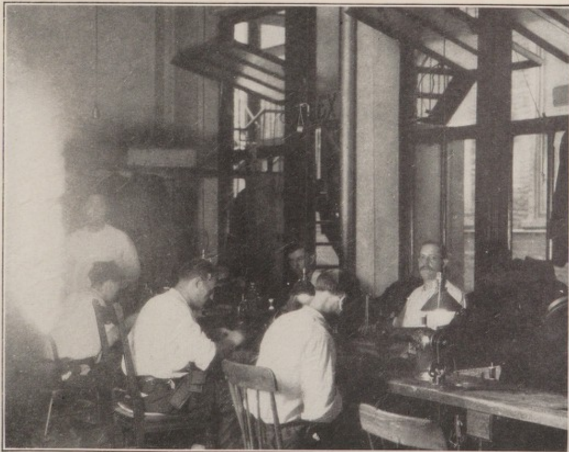
Fig. 2.—Glare effects from projecting filaments and low suspension in a shop with poor daylight illumination.
