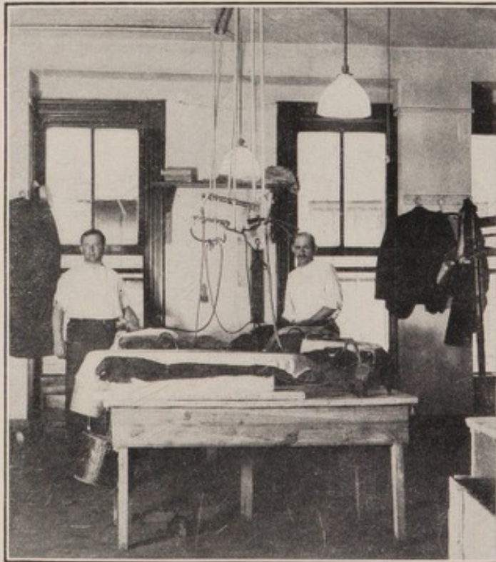
Fig. 10.—Pressing table, shop No. 11, with opal extensive bowl type reflectors, 250 watt tungsten lamps. The illumination was good. The lamps are well out of the visual field of the worker.
