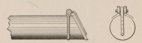
Fig. 33.—Automatic Outlet Gate.
