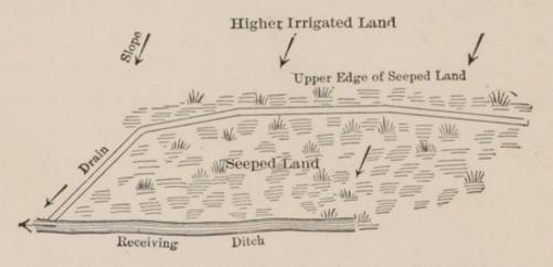
Fig. 45.—Location of Intercepting Drain in Seeped Land.
