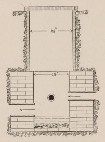
Fig. 30.—Silt Basin with Sewer-pipe Top.
