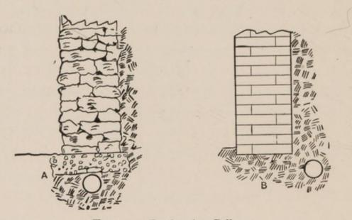
Fig. 39.—Drains for Cellars.
