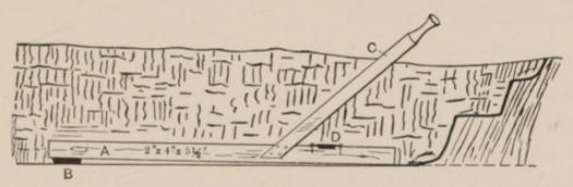
Fig. 25.—Grading by Drag Level.
