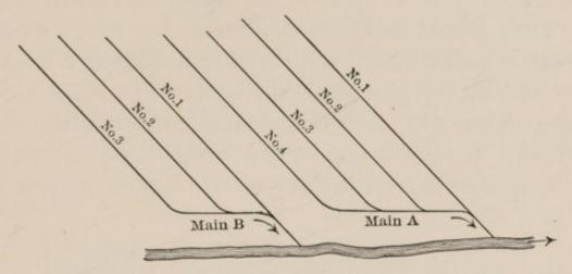
Fig. 16.—Modified Gridiron System.
