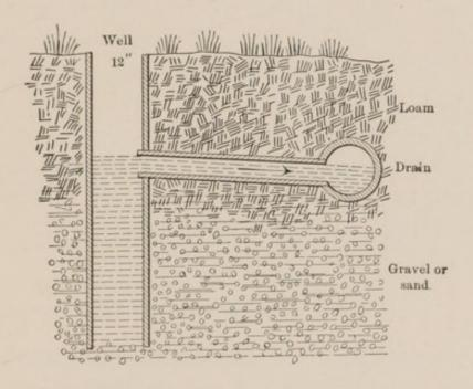
Fig. 46.—Well and Drain for Irrigated Land.
