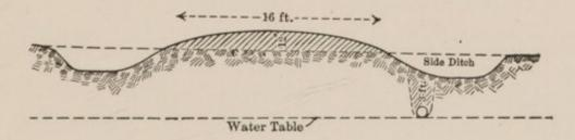
Fig. 41.—Section of Public Road with Underdrain.
