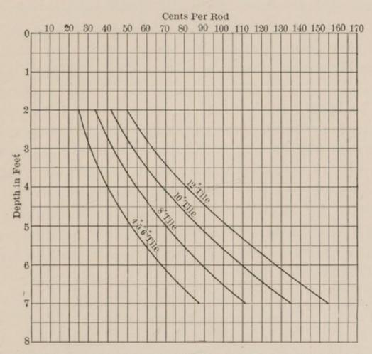
Fig. 38.—Diagram Showing Prices in Cents per Rod for Digging Trench and Laying Drain Tile.
