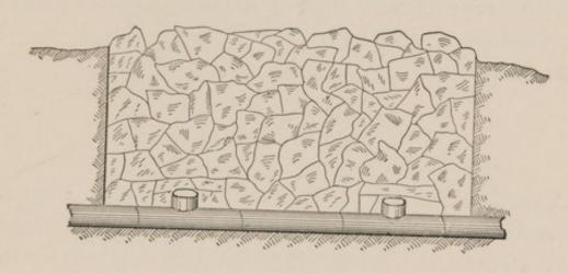
Fig. 31.—Surface Inlet to Tile Drain.
