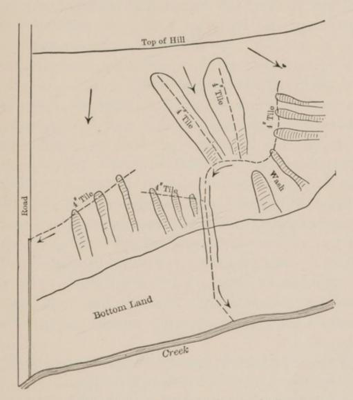
Fig. 43.—Tile Drains to Prevent Erosion of Hillsides.
