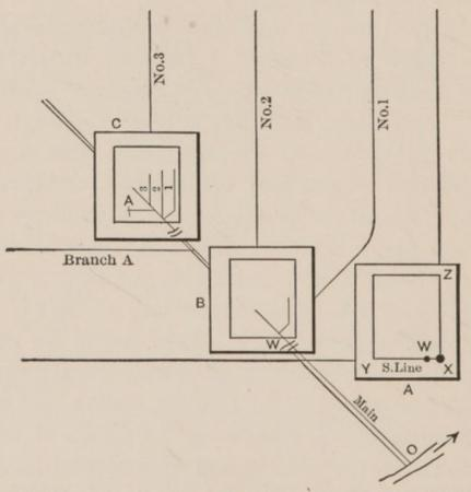
Fig. 36.—Mapping Drains on South Field with Plane-Table.
