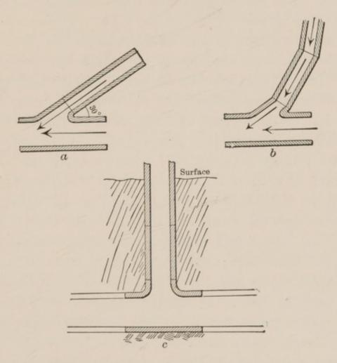
Fig. 28.—Horizontal and Vertical Junctions.
