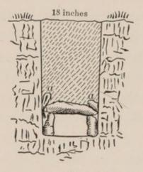
Fig. 10.—Drain Made with Thin Flat Stones.
