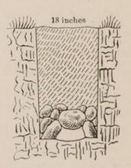
Fig. 11.—Cobble-stone Drain.
