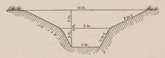
Fig. 7.—Ditch with Upper Half of Side Slopes less Steep.
