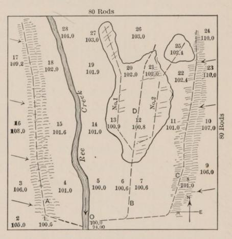
Fig. 20.—Preliminary Levels and Location of Drains on North Bottom Field.
