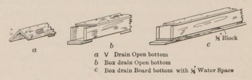
Fig. 9.—Plank Drains.
