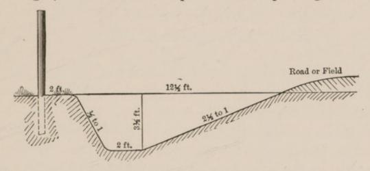
Fig. 8.—Fence Line Ditch. Excavations required  $15\frac{1}{3}$  cu. yds. to 1 rod.
