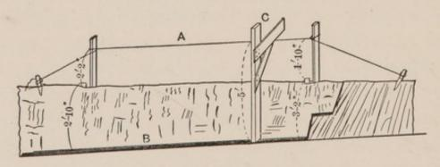
Fig. 24.—Grading by Line and Gage.
