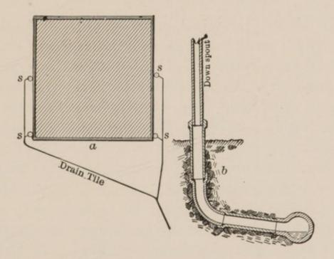
Fig. 40.—Tile Drain to Receive Roof Water from Barn.
