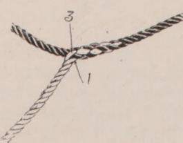
FIG. 145.—Side splice, fifth stage.
