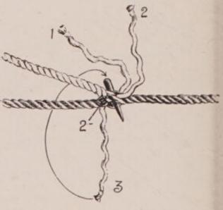
FIG. 142. — Side splice, second stage.
