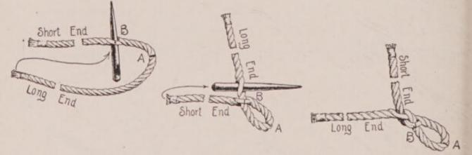
FIG. 147. — Rope halter. Forming the eye.
