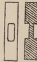
Fig. 120.—Method of cutting strips of plaster.
