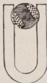
FIG. 22.—Diagram of Simple "Magneto," Generating an Alternating Current.
