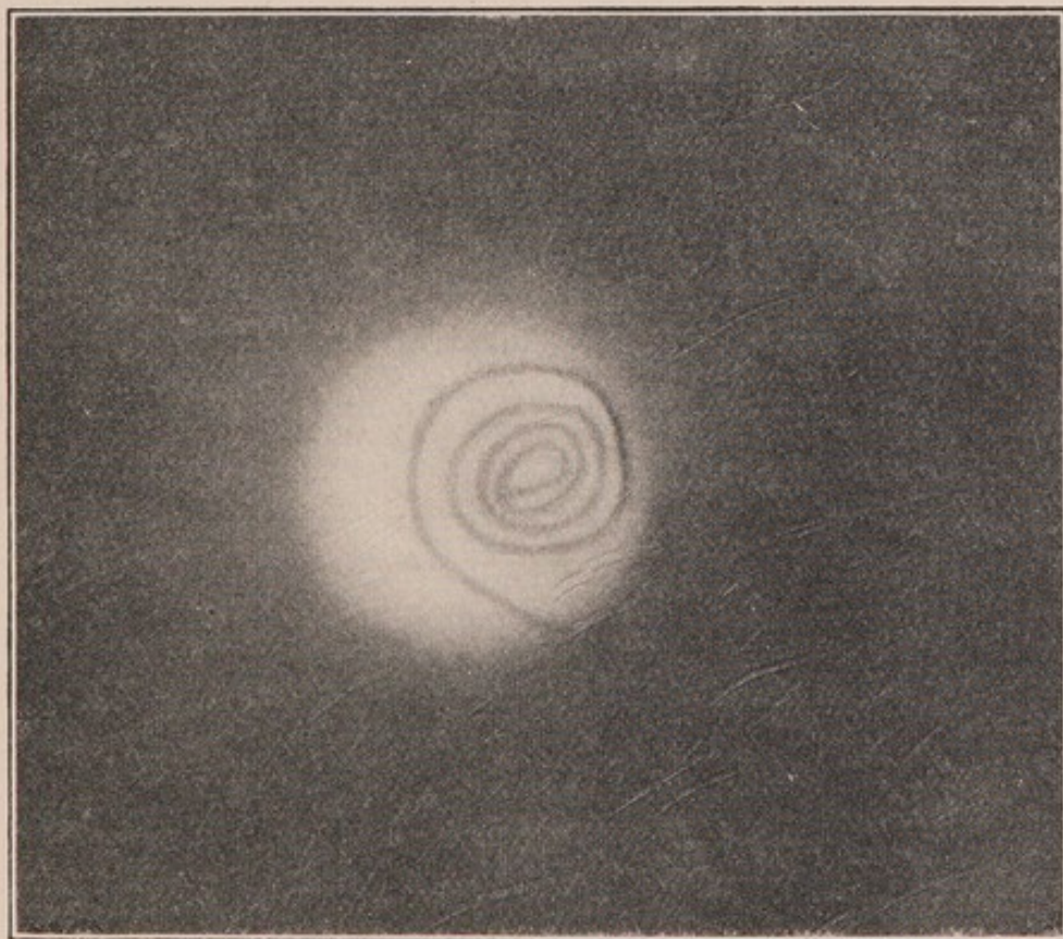
FIG. 17.—Radiograph of wire spiral by pitchblende residue ( \beta and \gamma rays). Exposed 7 days.
