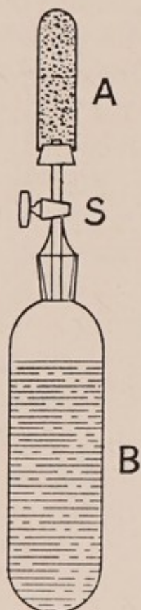
FIG. 23.—Method of showing fluorescence due to the \alpha radiation from radium emanation.
