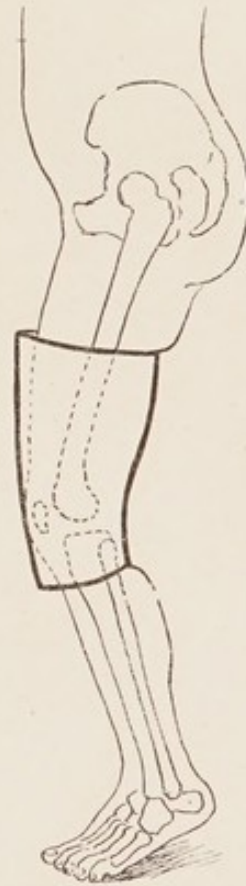
Fig. 85. Wrong knee splint. Demonstrating cast cutting into flesh.
