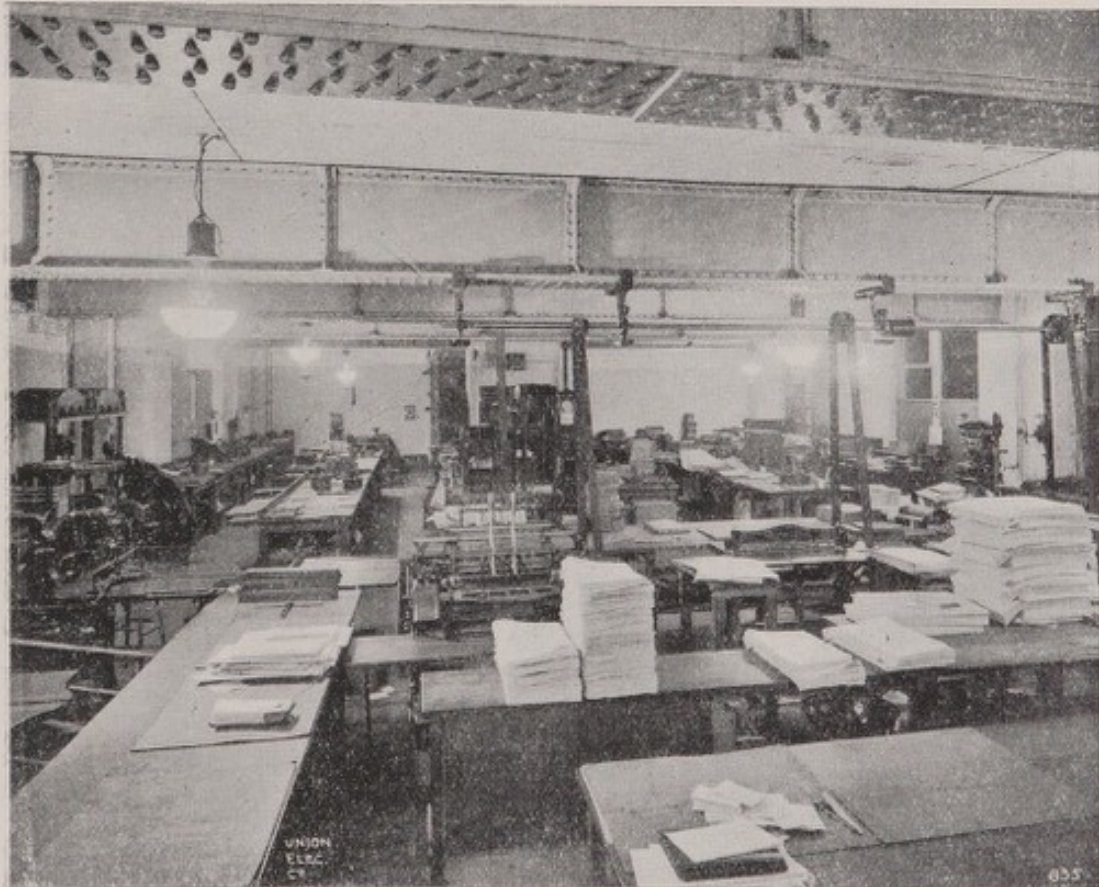
FIG. 163.—Semi-indirect (Union) arc lighting in the paper room of a printing-works.
