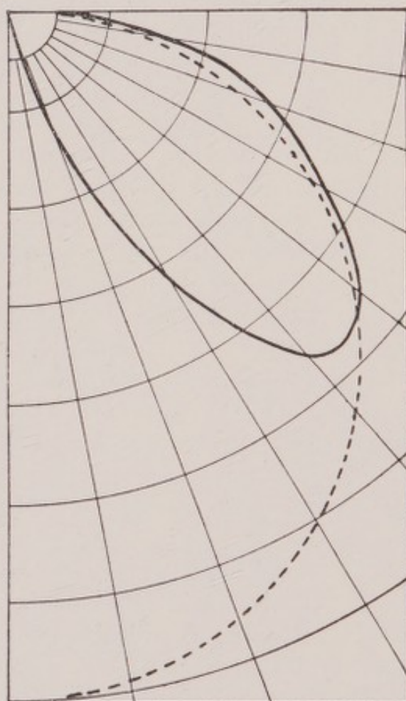
FIG. 36.—Curve showing maximum distribution of light from ordinary d.c. arc (Trotter).
