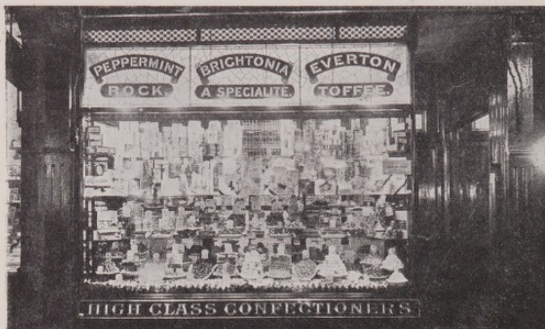
FIG. 173.—Window lighted by concealed lamps—a much better method.
