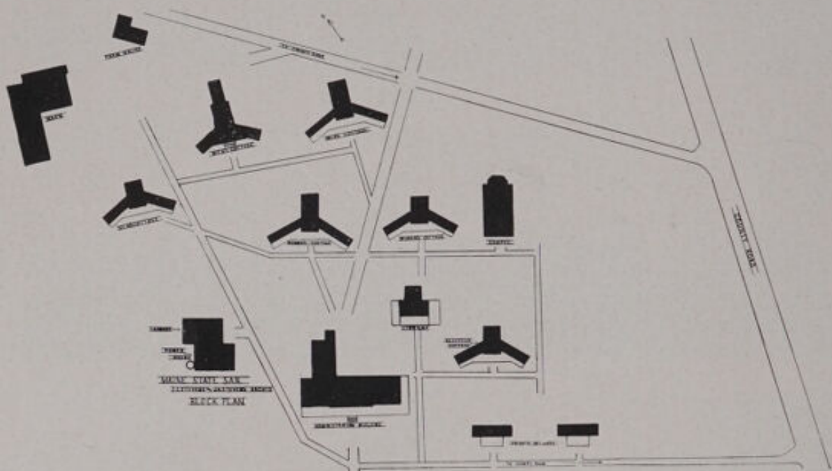
No. 11.—Maine State Sanatorium, Hebron, Me. T. C. STEVENS AND J. H. STEVENS, ARCHITECTS. VIEW AND BLOCK PLAN SHOWING METHOD OF GROUPING PAVILIONS IN THE REAR OF THE ADMINISTRATION BUILDING AND POWER HOUSE. CAPACITY, 100 PATIENTS. ESTIMATED COST, $150,000. (See illustrations 23 and 38 for further description of this institution.)
