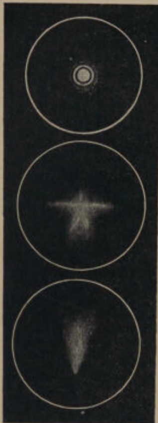
FIG. 99.—Appearance of coma and astigmatism together.
