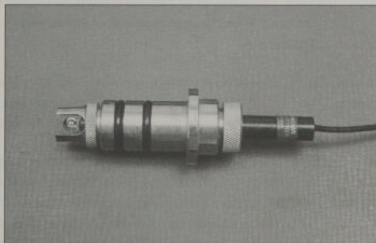
pH electrode for insertion in fermenter wall
