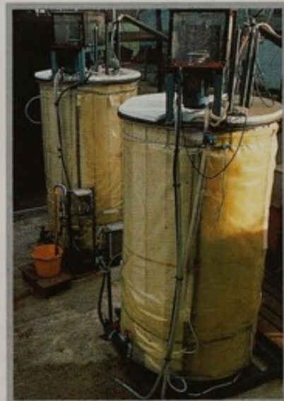
C oncentrations of odour and ammonia are analysed and pilot scale studies of the aeration of pig slurry are carried out at the Silsoe Research Institute to develop odour control techniques.
