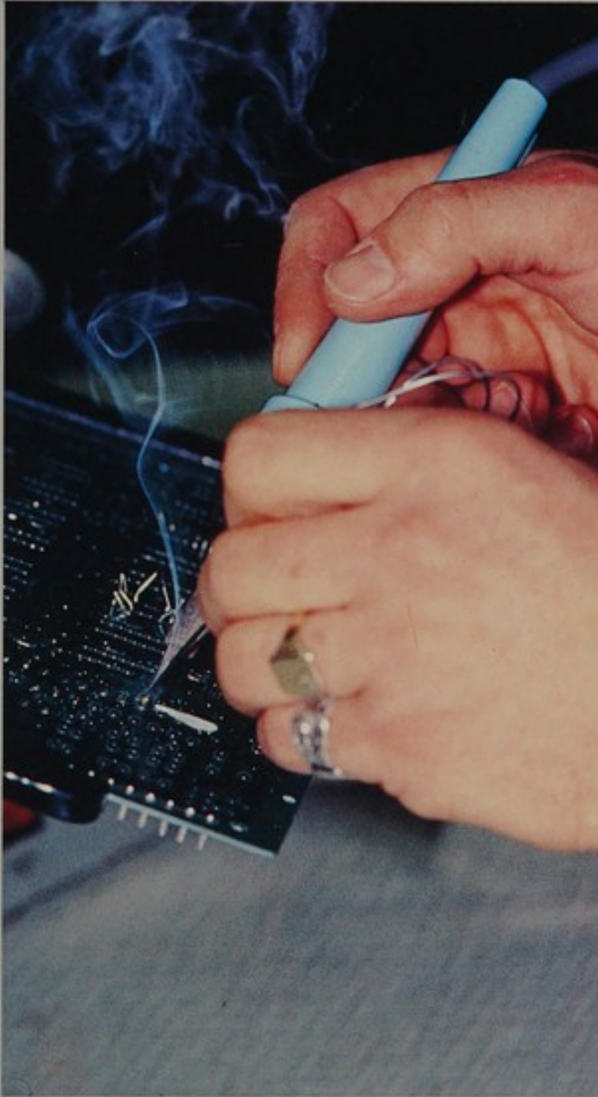
Colophony fumes - the absence of any extraction results in operator breathing in the fumes
