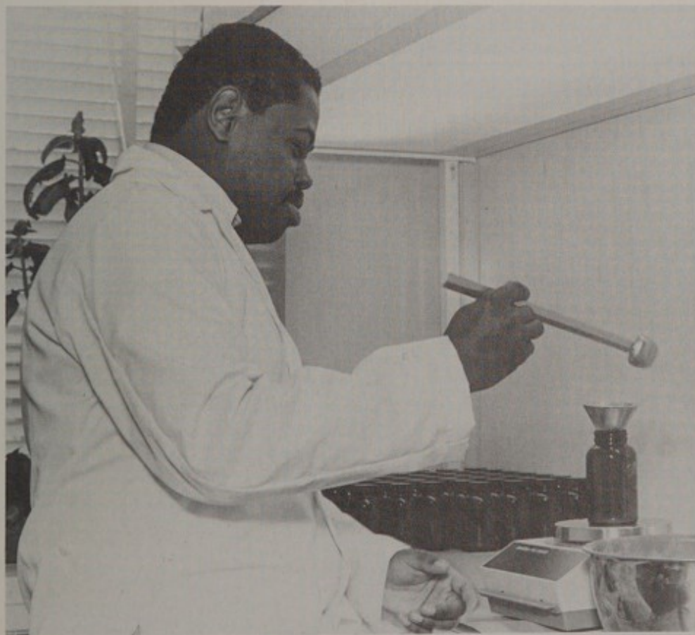
Powdered SRM's are packaged by weight. John Savoy uses a balance to assure the correct amount in each bottle.
