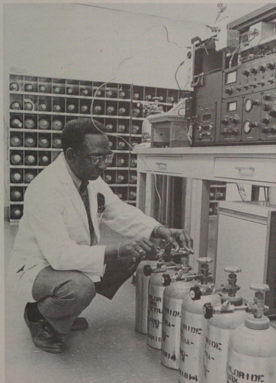
Research chemist Bill Cuthrell prepares to analyze the concentration of a proposed gas SRM.
