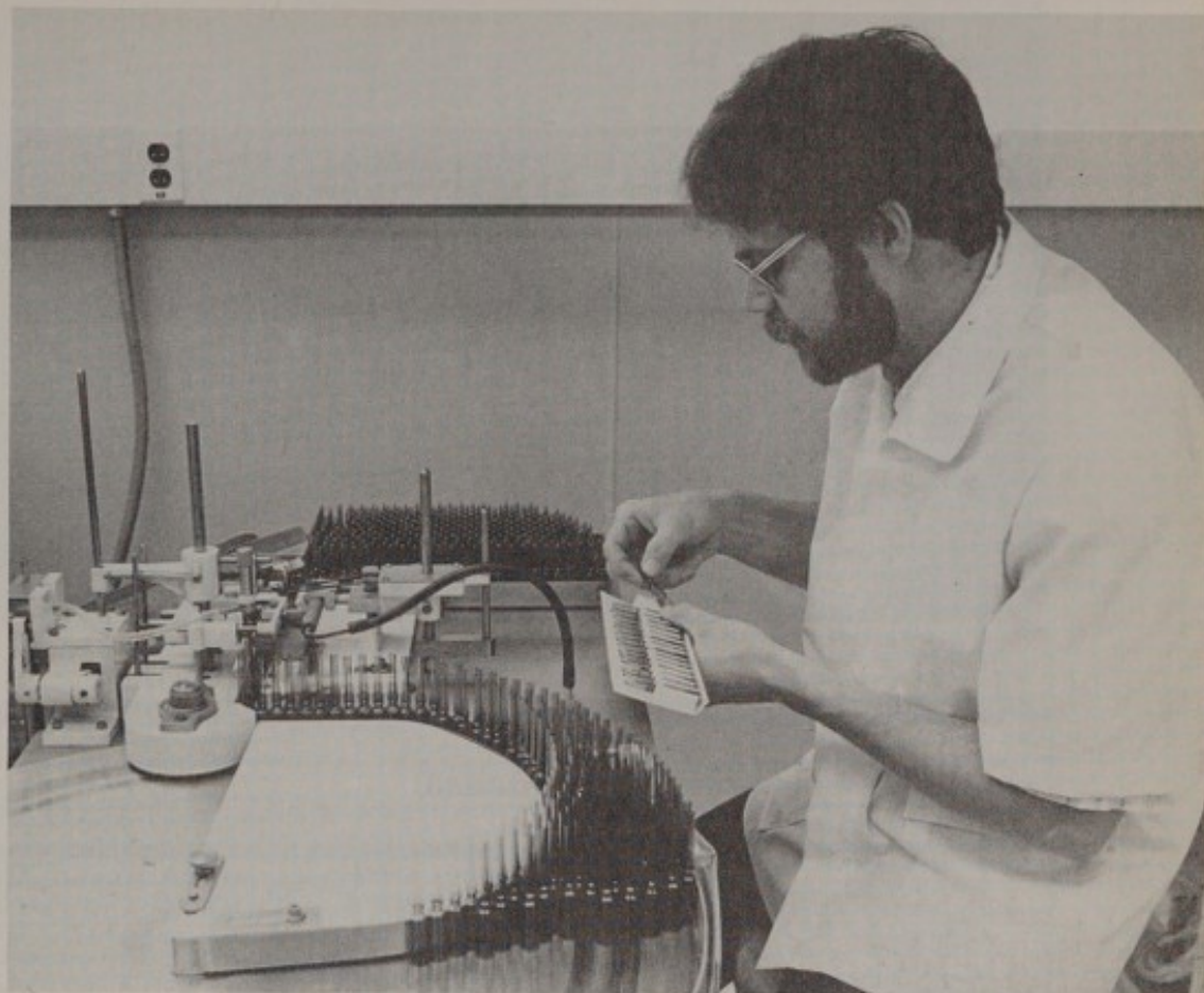
Dale Friend operates equipment that fills and seals ampoules used for various liquid SRM's.
