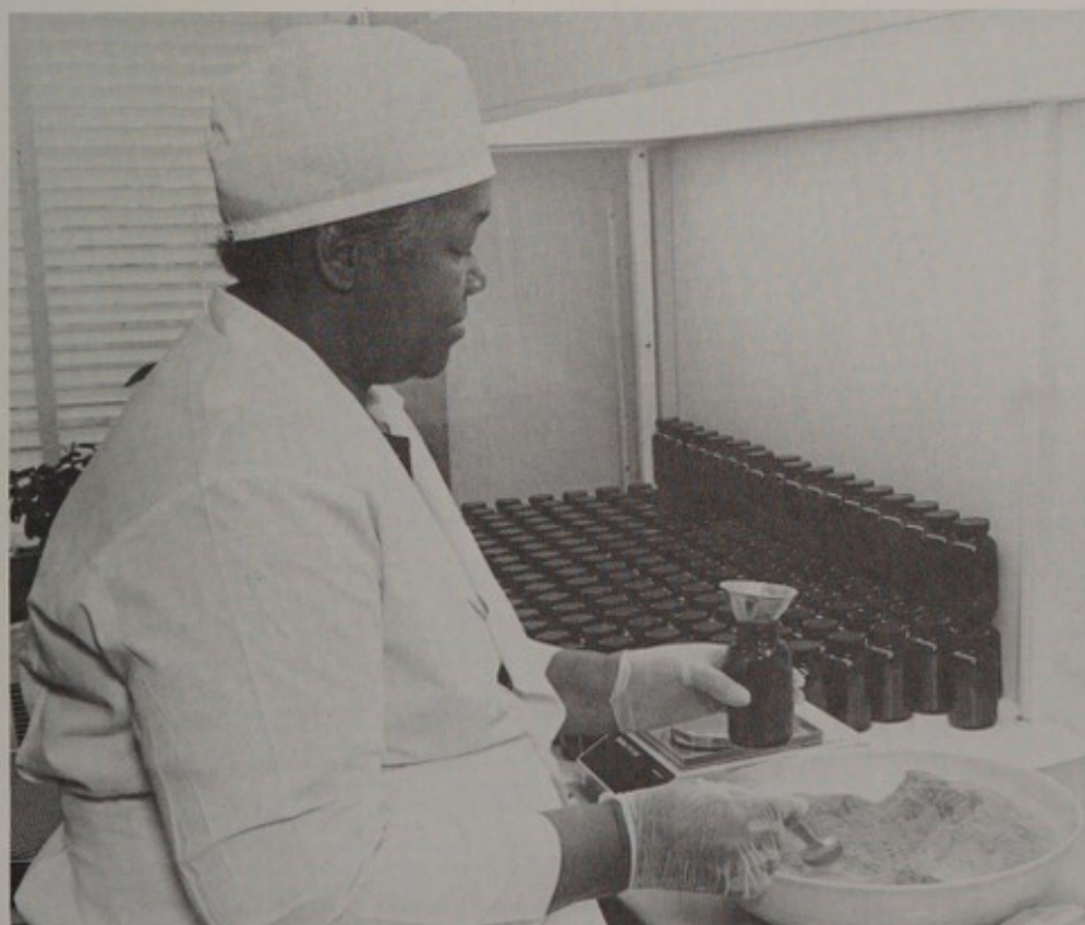
Many SRM's are certified as bulk material and then packaged by weight into individual containers, as Helen Tyler is doing with this powdered SRM.
