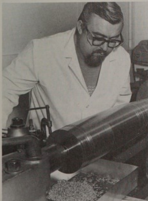
Frank Mills controls the chipping of a titanium alloy that will be ground, sieved, and blended to insure high homogeneity before analytical testing for certification.
