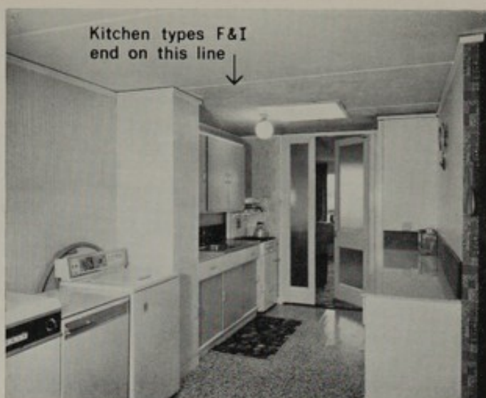
15 Kitchen type H. Kitchen types F & I finish on the line shown. Whilst kitchen type I gets direct daylighting from a similar rooflight, kitchen type F relies entirely on borrowed lighting through the glazed door and panel.
