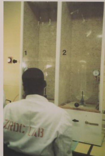
Condom testing, Zimbabwe Regional Drugs Control Laboratory (Appendix 4B)
