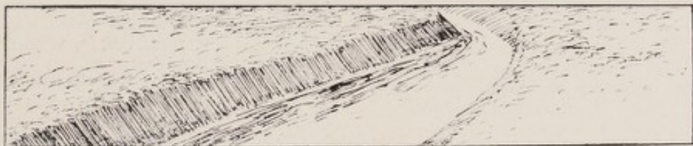
Figure 2. — The breeding-place of Anopheles minimus var. flavirostris has been thoroughly exposed to the sun by cutting all vegetation and having the banks of the stream clean-cut at 45° inclination with straight borders along the water level.
