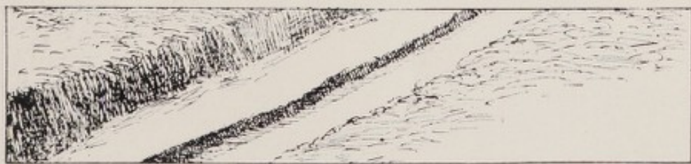
Figure 3. — Breeding-place of Anopheles minimus var. flavirostris , showing ditch built at about the middle of the stream bed along its course, thus allowing all of the water to flow through the ditch.
