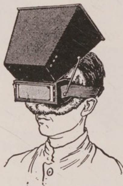
Fig. 97. Dessane's fluoroscope elevated to the top of the head after the fluoroscopic examination has been made permitting the operator to see by ordinary light without losing the sensibility of the retina because of a ruby glass which automatically drops in front of the eyes as the fluoroscope is elevated.
