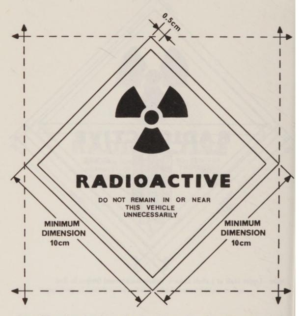
Note—When dimensions larger than the minimum dimensions shown are used, the relative proportions must be maintained
