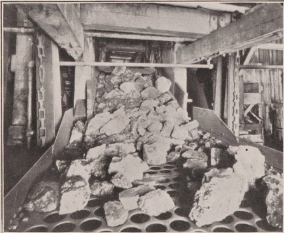
FIGURE 9.—PRIMARY SHAKING SCREEN.
