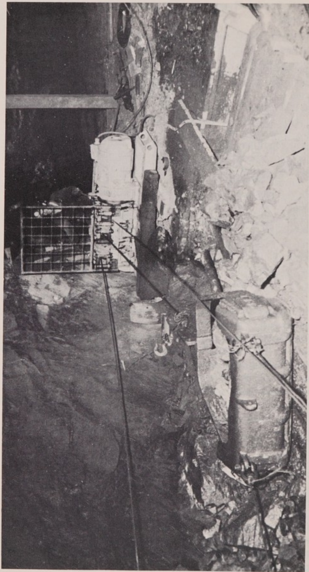
Miner operating electric tugger in slushing operation. (Courtesy of The Homestake Mining Co., 1963.)
