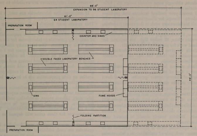
FIGURE 18.—Layout for a conventional teaching laboratory with double-faced benches.
