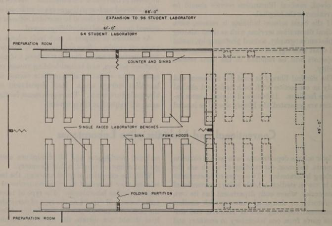
FIGURE 17.-Layout for a conventional teaching laboratory with single-faced benches.
