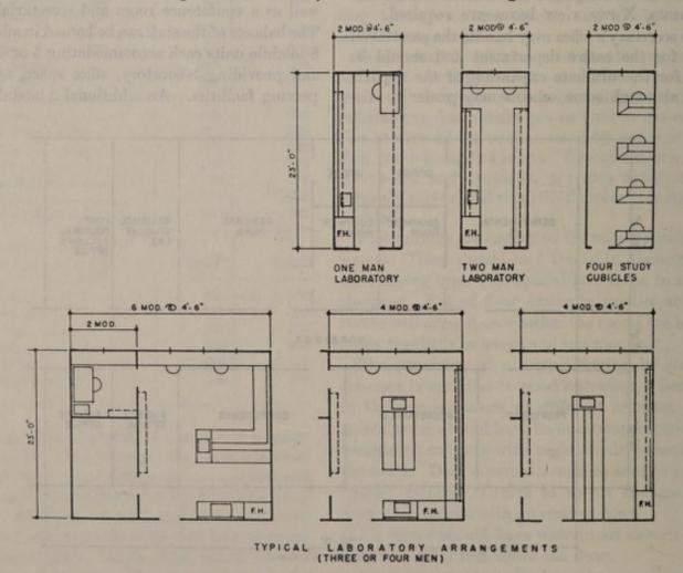
FIGURE 11.-Layouts for research laboratories.
