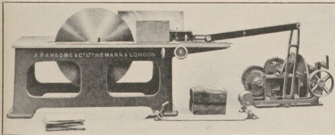
FIG. 36.—Mechanical Feed. The necessary guards for saw and gearing, etc., are not shown. (Messrs. A. Ransome & Co., Ltd., Newark; Bisset's Patent.)
