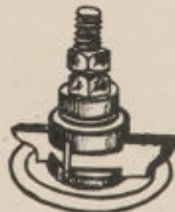
FIGS. 62, 63 and 64.—Types of Spindle-Moulder Cutter-Blocks.
