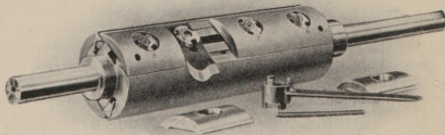
FIG. 51 D.—Segmented Circular Block with Moulding Irons fitted. (Messrs. Wilson Bros., Leeds.)
