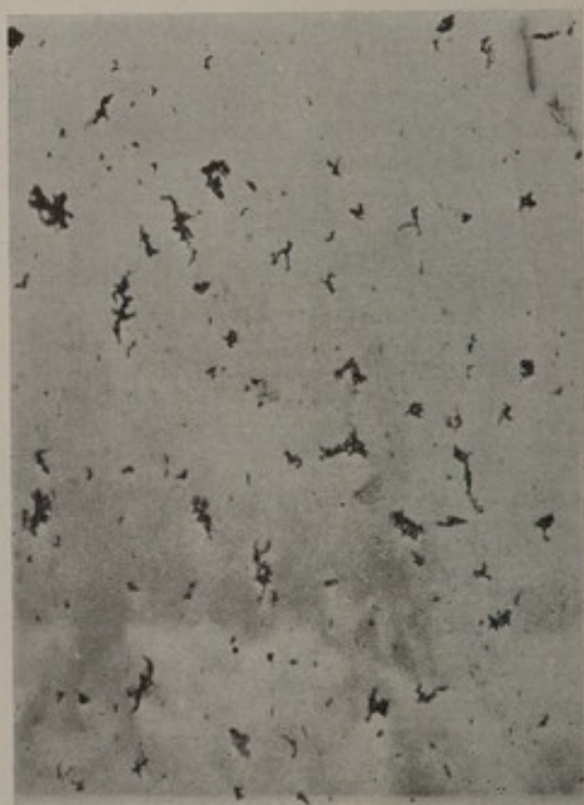
FIG. 7. GRINDING CARD ROLLERS. (WILLOWED WOOL. 119 MGMS. DUST.) MAGNIFICATION \times 75 .
