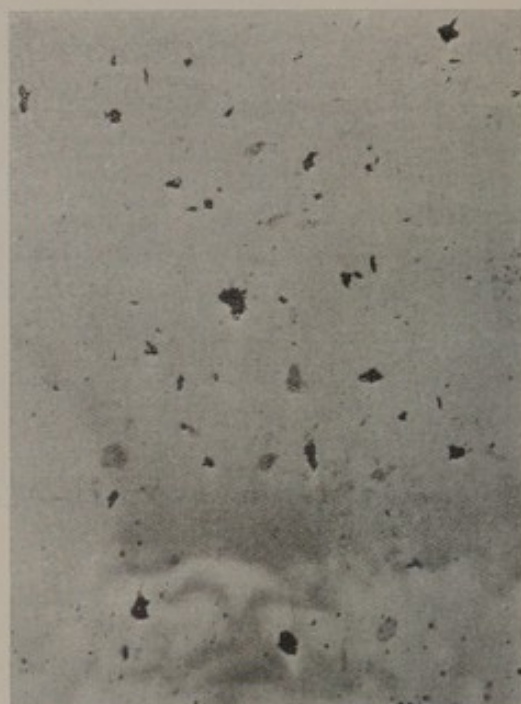
FIG. 5. GRINDING CARD CYLINDERS AFTER VACUUM CLEANING. (40 MGMS.) MAGNIFICATION \times 75 .
