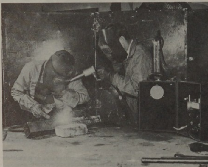
Industrial hygienist samples welding fumes with an electrostatic precipitator.
