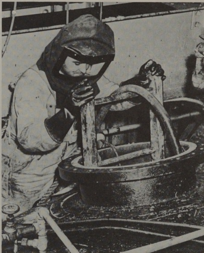
An air-supplied helmet and life-line protect the worker who must clean the interior of a stripping tank in a synthetic rubber plant.
