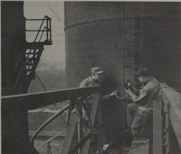
Public Health Service engineer taking static pressure reading for purpose of calculating air flow at Donora.
