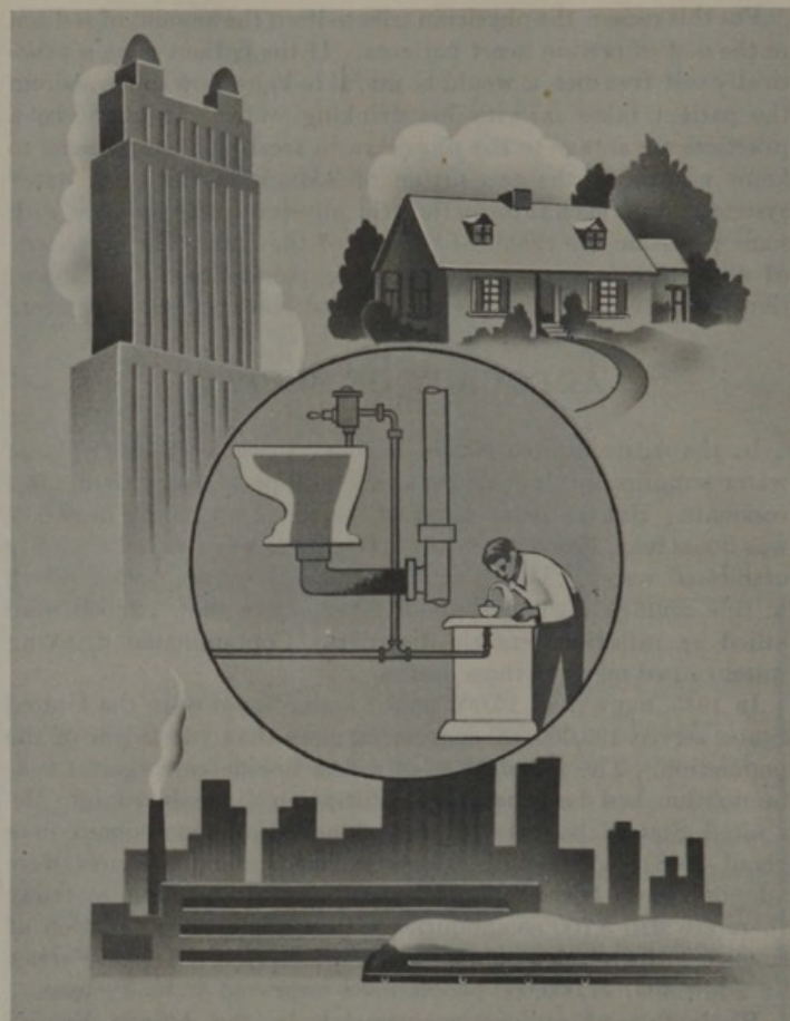
Faulty plumbing in office, home, factory or school is a weak point where germs may enter the water supply. Drinking water must be protected all the way from the reservoir to the tap.
