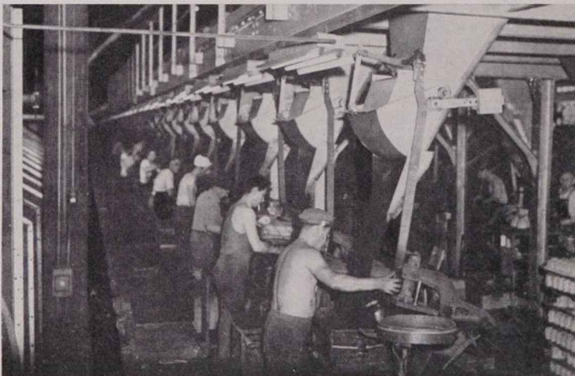
Figure 3.—Line of machine molders. Molding sand is provided by an overhead conveyor system. Finished molds are taken to a central pouring area by the conveyor directly behind the molders.
