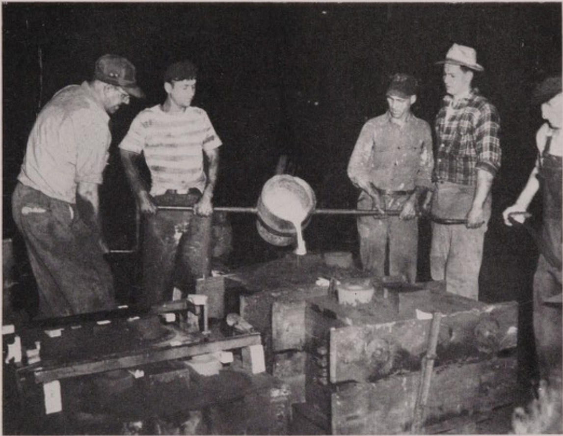
Figure 4.—Manual pouring of hot metal into floor molds.
