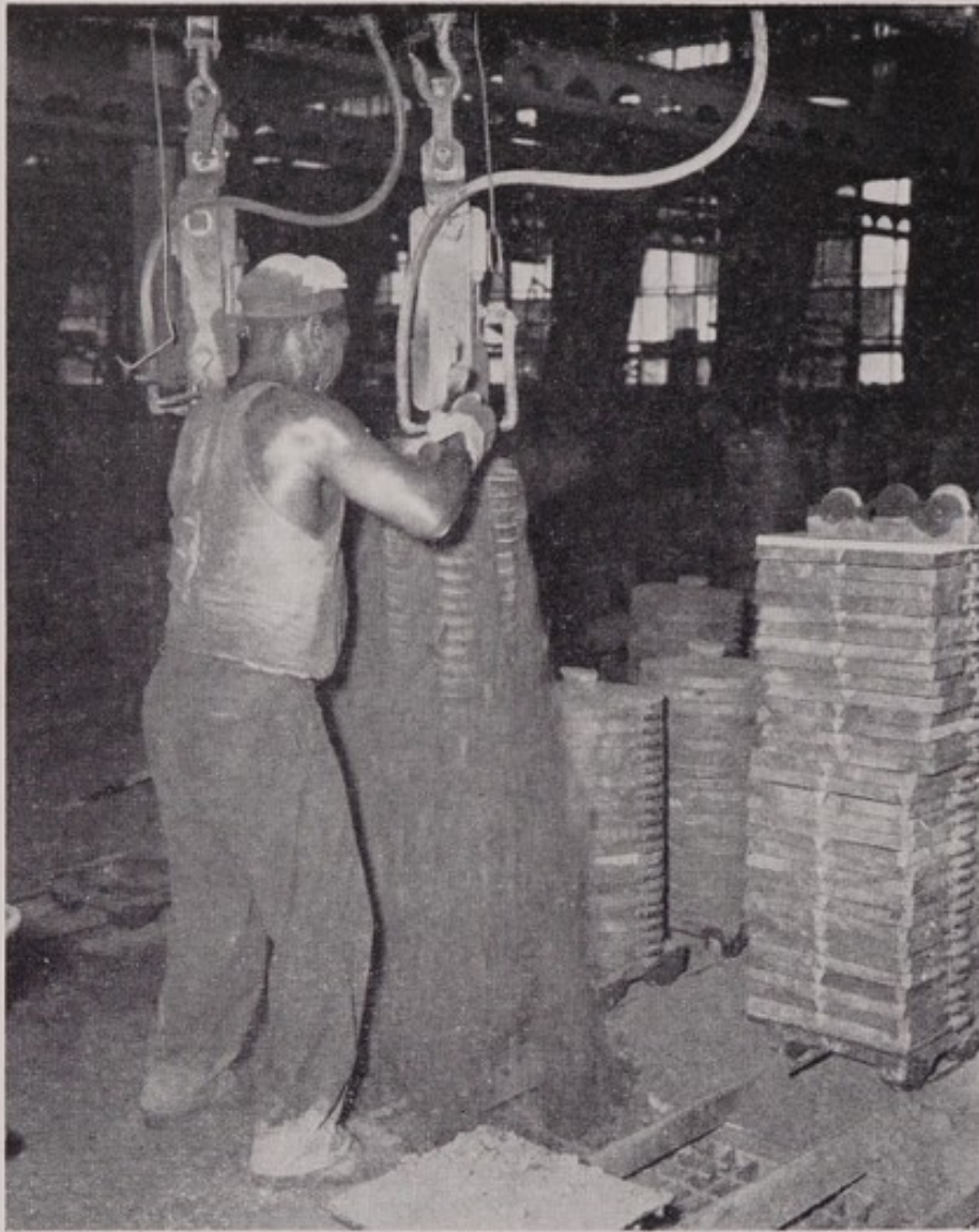
Figure 11.—Shakeout of castings using a pneumatic vibrator hoist. Sand falls through grillwork in floor onto conveyor belt which carries it to the sand conditioning unit.
