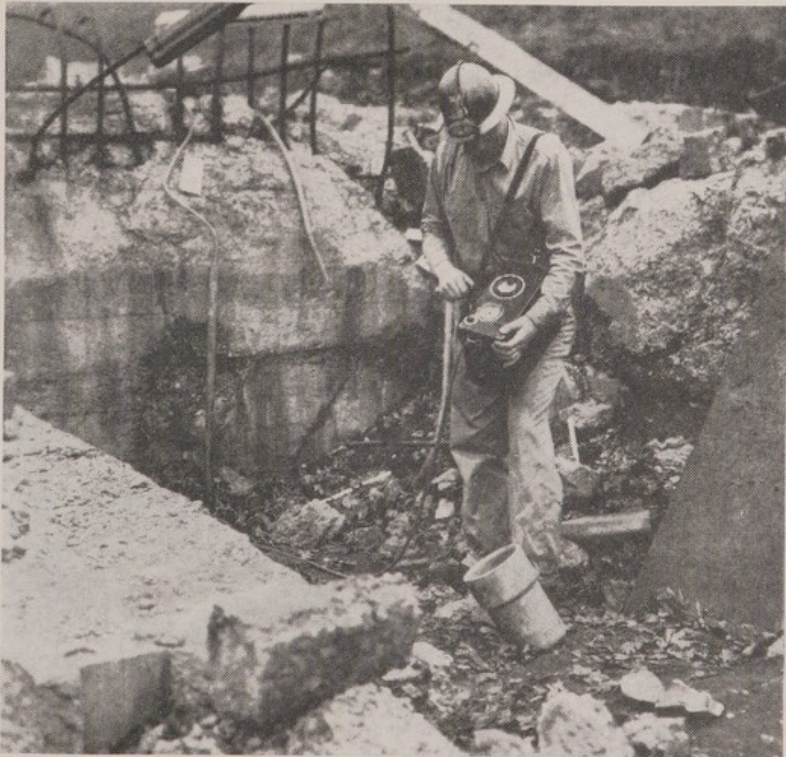
FIGURE 11.—Carbon monoxide indicator (hand-type) calibrated to register carbon monoxide concentrations within the range of 0.005 to 0.15 percent.
