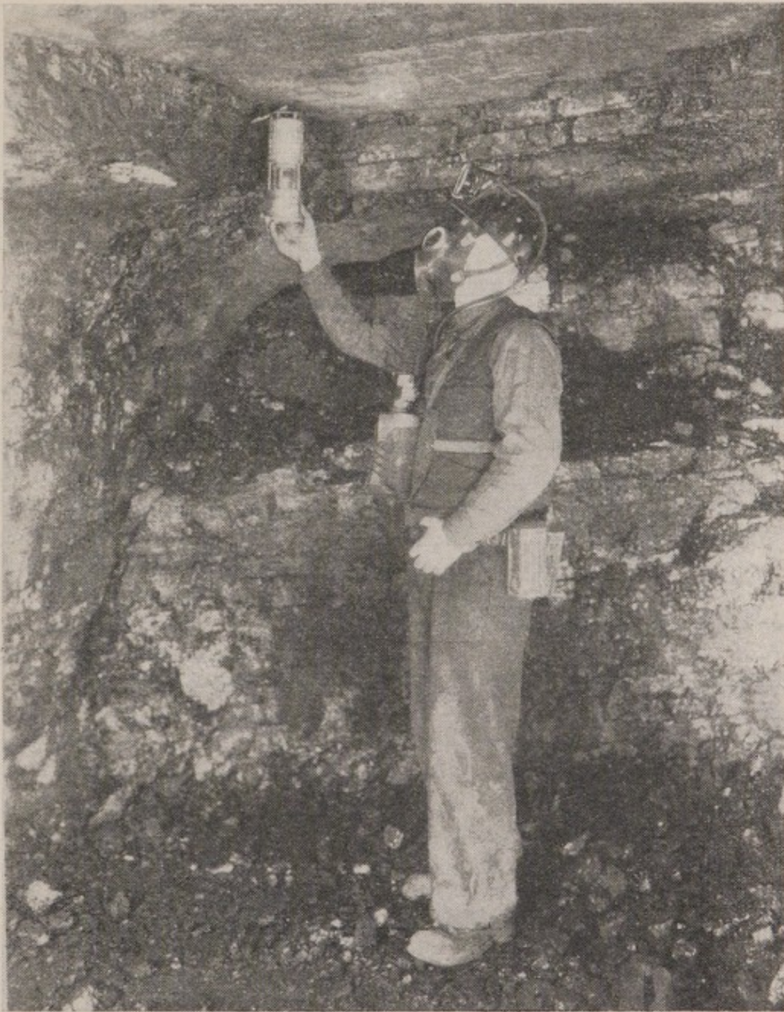
FIGURE 1.—Miner wearing “all-service” gas mask and testing with flame safety lamp for methane gas and oxygen deficiency.
