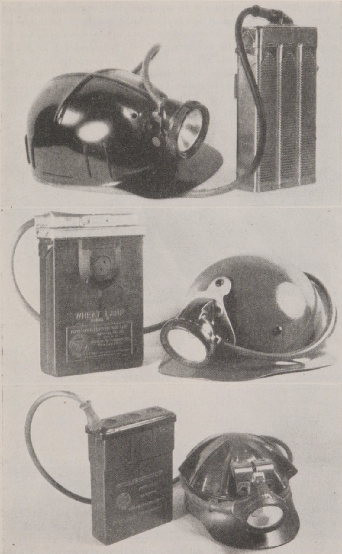
FIGURE 7.—Permissible Electric Cap Lamps with Protective Cap.
