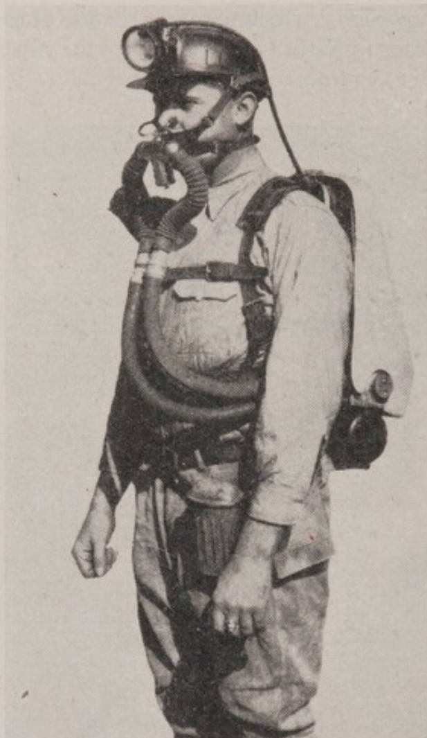
FIGURE 5.—A 2-hour oxygen breathing apparatus.
