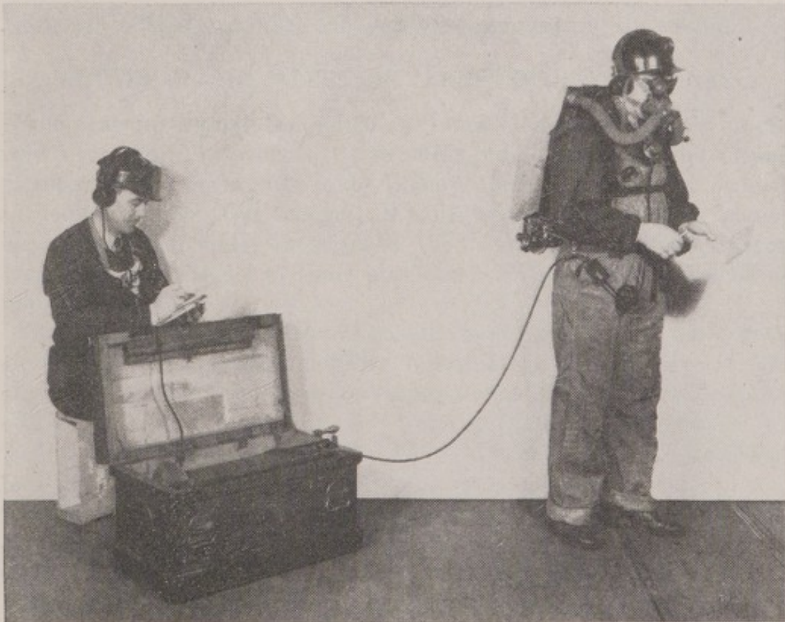
FIGURE 13.—Portable telephone life line unit assembled for use by the apparatus wearer and the listener at the fresh-air base.
