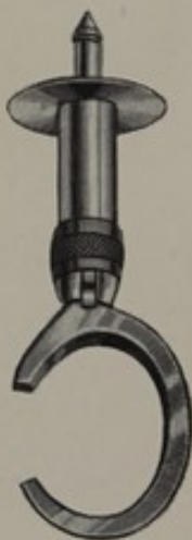
Fig. 40.— Mechanical " C " Hook.
