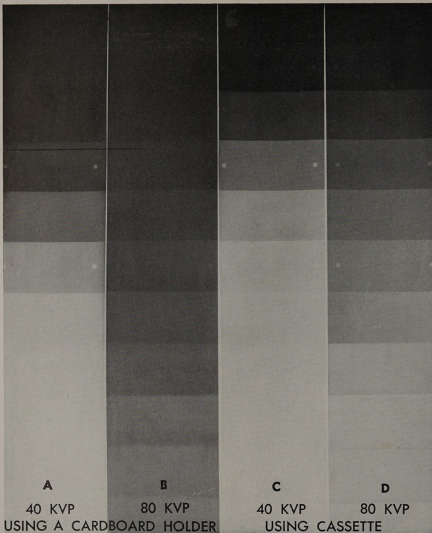
Figure 82. The effect of cardboard holders and intensifying screens on contrast.
