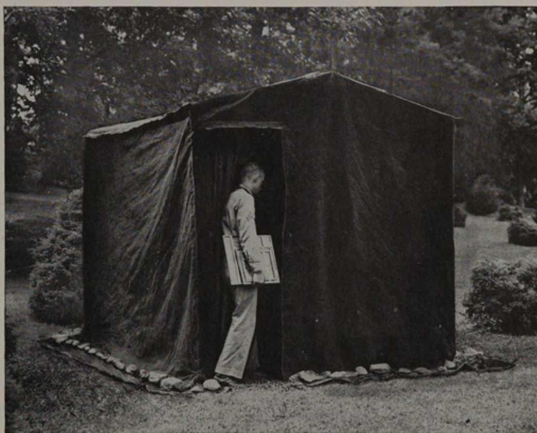
Figure 62. Item 96175. The adjustable inner curtain set back with auxiliary drapes extending to provide the labyrinth as needed when the tent is to be used for film processing.
