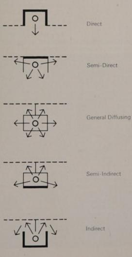
108. As is the case in the design of daylighting, varying the proportions of direct and indirect artificial light has a marked effect upon the character of an interior.
