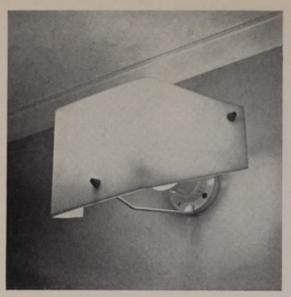
A simple fitting moulded from acrylic plastic sheet, and designed within the Regulations concerning cut-off and brightness for use with a 60 watt tungsten lamp on walls where pupils may at times have to work with their backs to the main windows.
