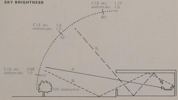
Diagram 3: Direct and indirect daylighting The total daylight factor at any point in a room is made
