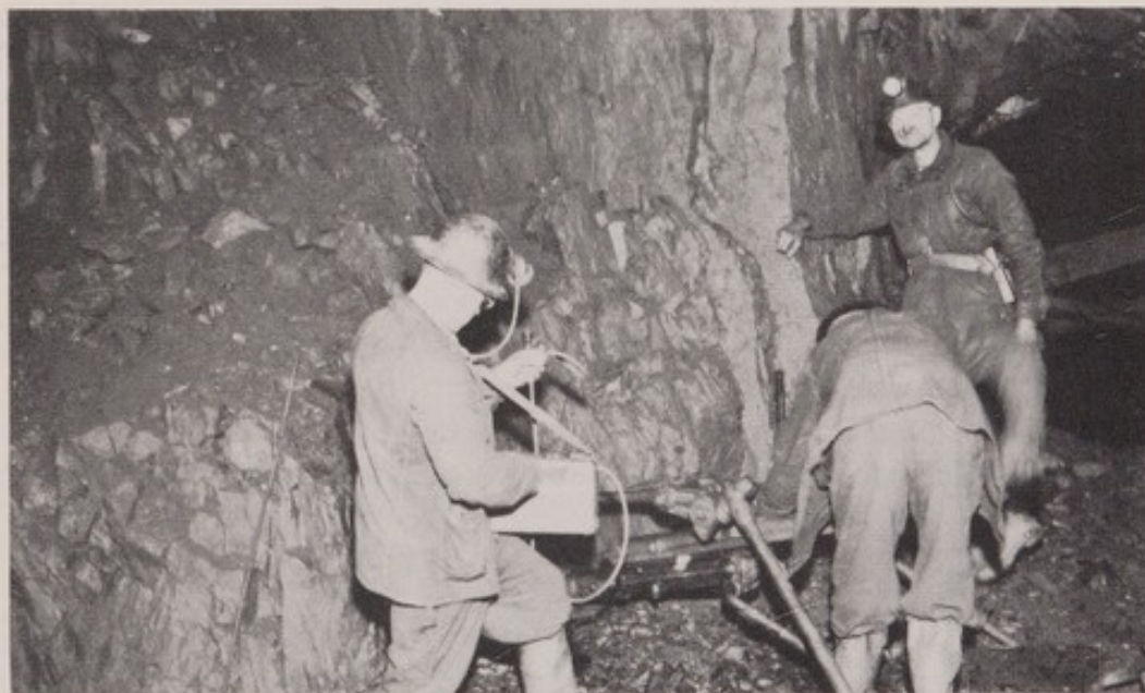
FIGURE 5.—Dust Sampling With Midget Impinger.
