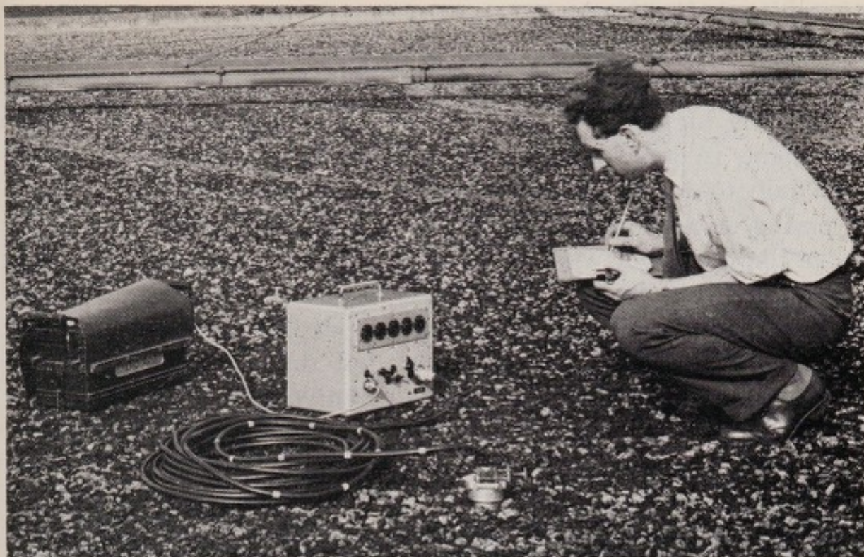
17. Measuring the moisture content of a percolating filter by neutron scattering
