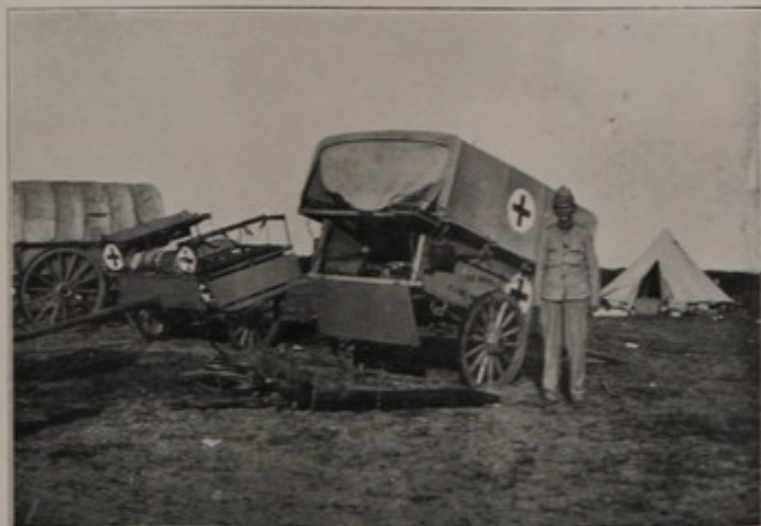
MANDER'S FLYING AMBULANCE. (That to the right carries three men lying down; that in the centre is for sitting-up cases only.)
