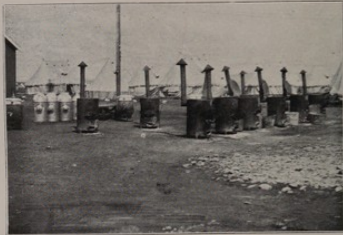
SOYER'S STOVES FOR BOILING DRINKING WATER, AND AYMARD'S STERILISERS No. 20 GENERAL HOSPITAL.
