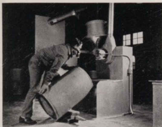
Filling the hopper, situated on the floor above the feeder. Dust extractor (Omega) is fitted.
