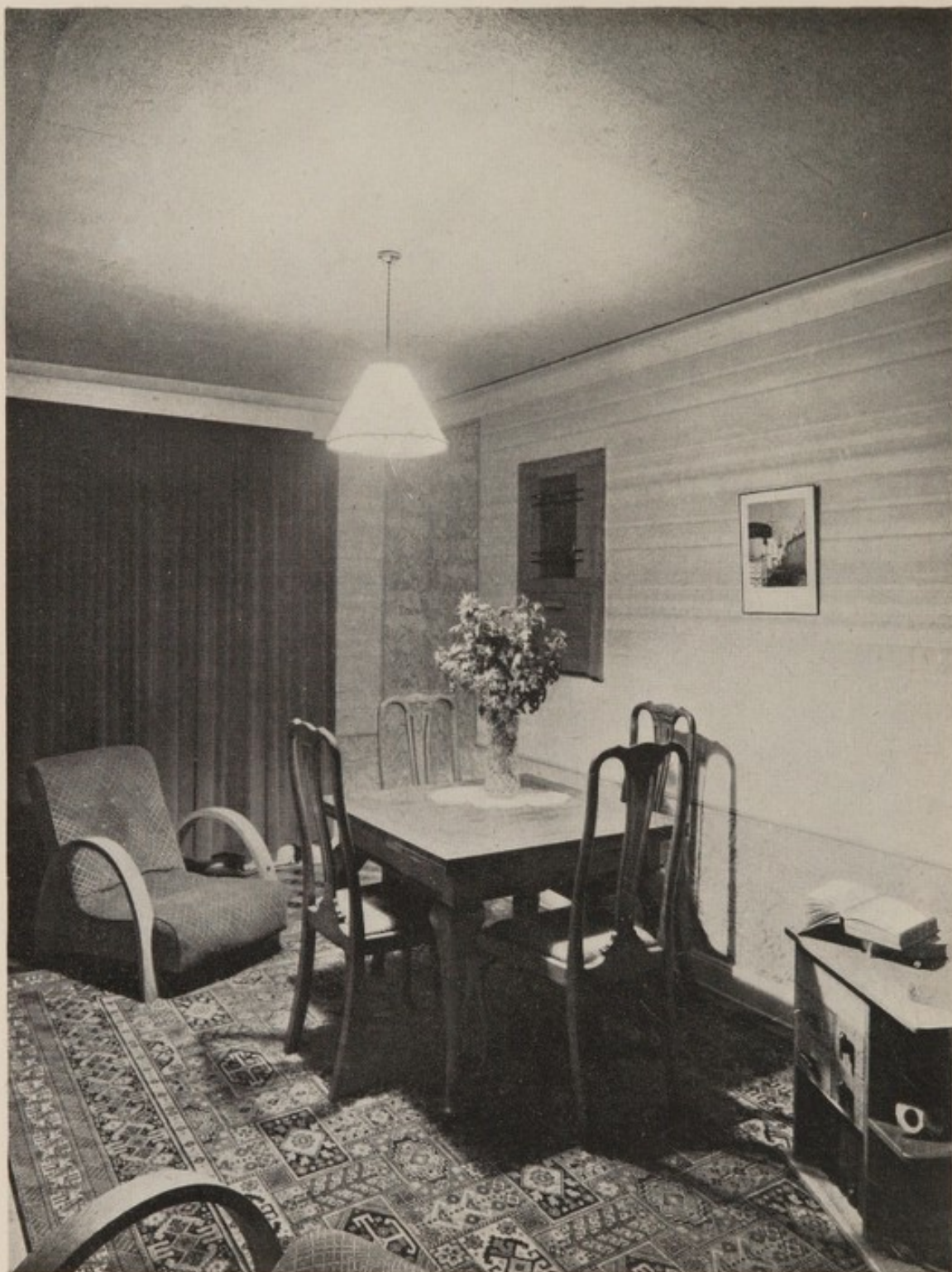
PLATE 2. A SEMI-DIRECT LIGHTING FITTING, WITH MOST OF THE LIGHT GOING DOWNWARD
