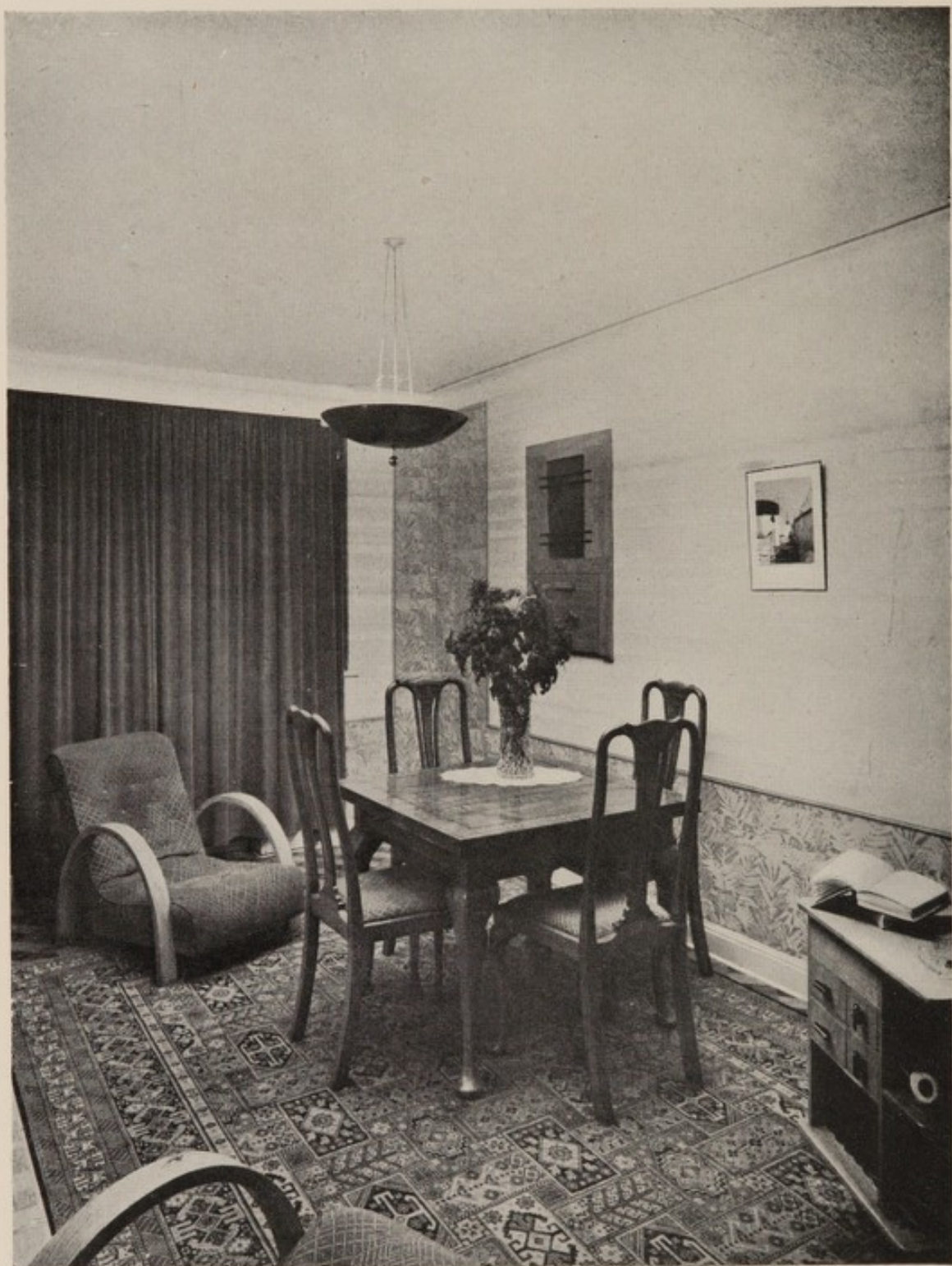
PLATE 4. AN INDIRECT FITTING, WITH ALL THE LIGHT DIRECTED UPWARD
