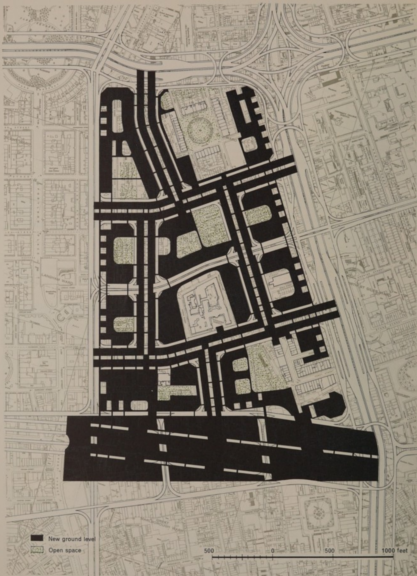
196 The design for partial redevelopment showing existing buildings to be retained at ground level and, in black, the raised deck on which the new building would be constructed.
