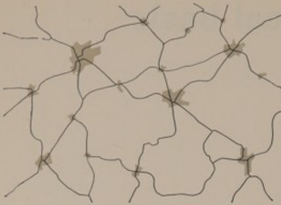
43 The inherited road system. Direct links from town centre to town centre, forcing all long-distance traffic to pass through the middle of towns.
