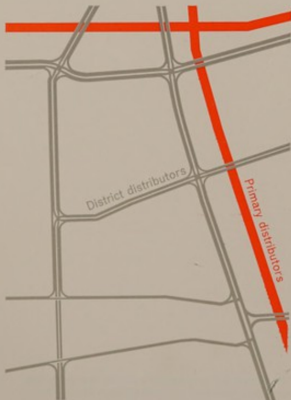
190 The theoretical arrangement of primary and district distributors.
