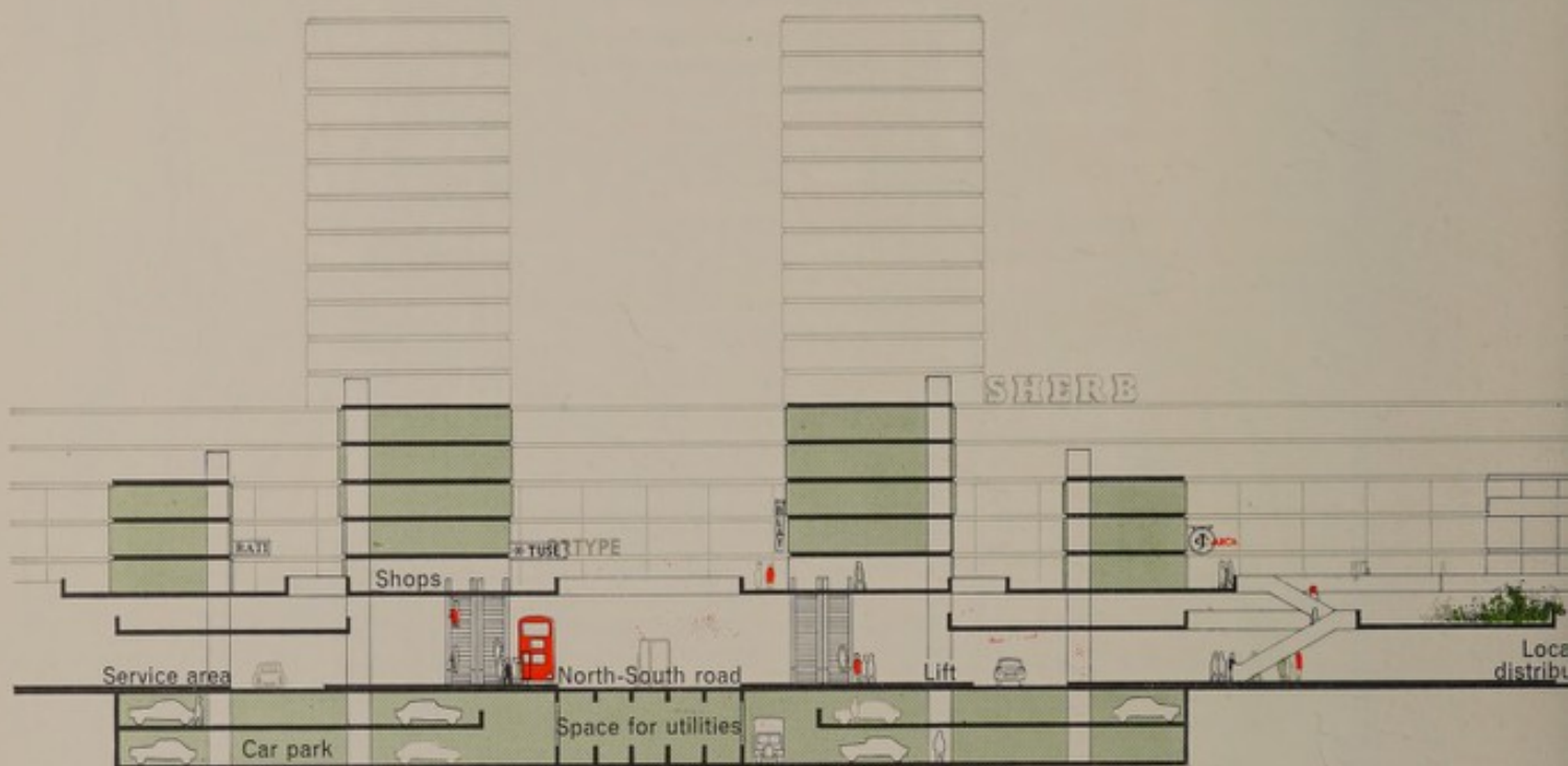
183 Design for complete redevelopment. This sectional view (for the location of the section see AA on Figure 182) shows the north-south zig-zag road on the left-hand side, with local shops above it at the new ground level. Pedestrian ramps and walkways link down to the open space on the right-hand side of the section.
