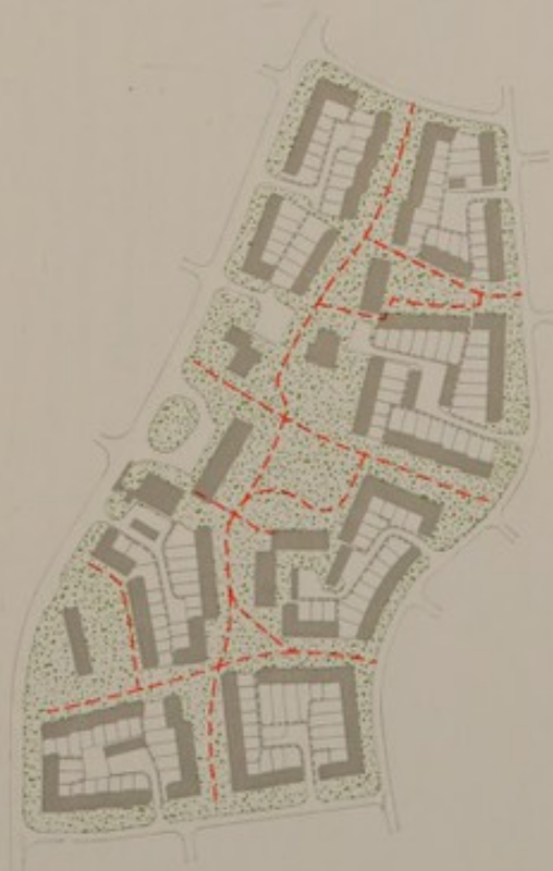
62 The Radburn principle in practice. A layout from Sheffield.
