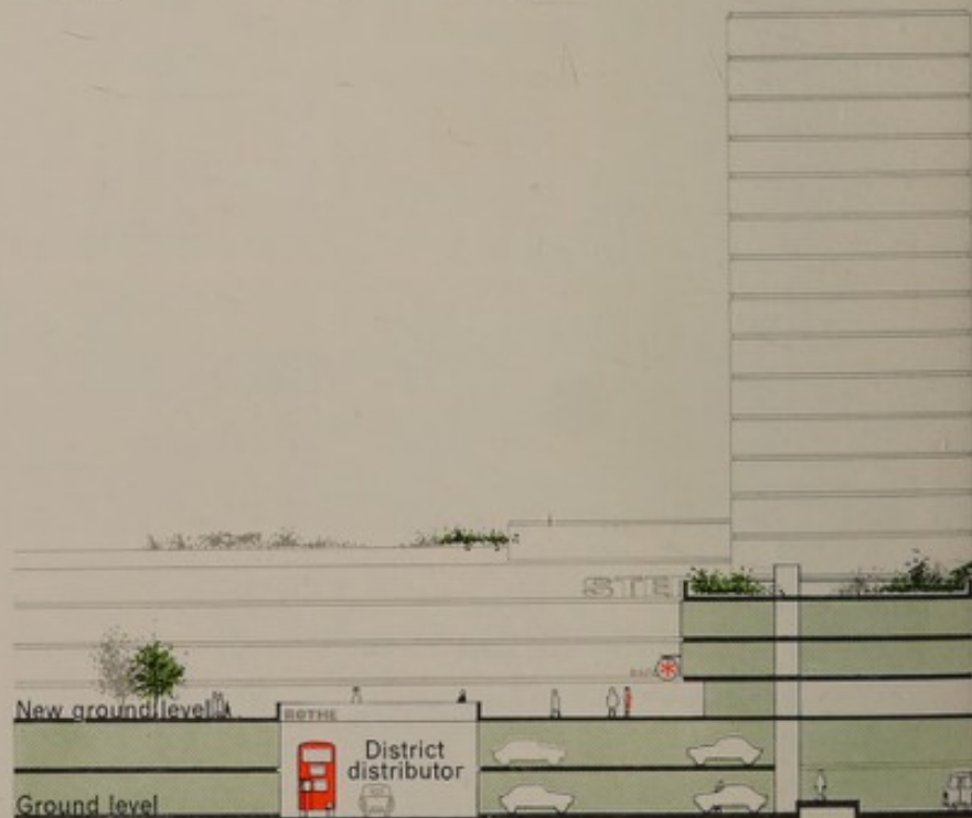
198 Scheme for partial redevelopment. Section through Oxford Street shopping centre, showing the district and local distributors and access road at ground level, and the shops at the 'new ground level' above (section DD on Figure 197).
