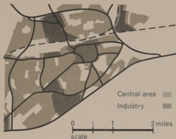
215 Basingstoke. This is the first plan, based on conventional ring roads, which was tested as the basis for expansion and redevelopment. It may be compared with Fig. 216 which shows the plan finally adopted after full analysis of traffic movement and environment.
