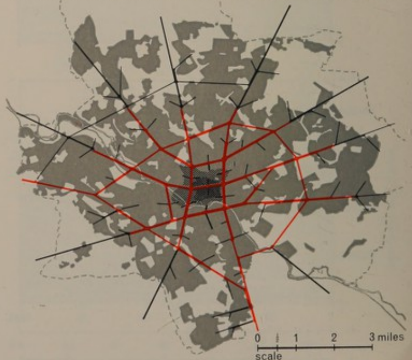
121 The theoretical intermediate network which would meet about 40% of the potential demand for travelling to work by car in the central zone. The distributors shown in red would need to be built to motorway standards.
