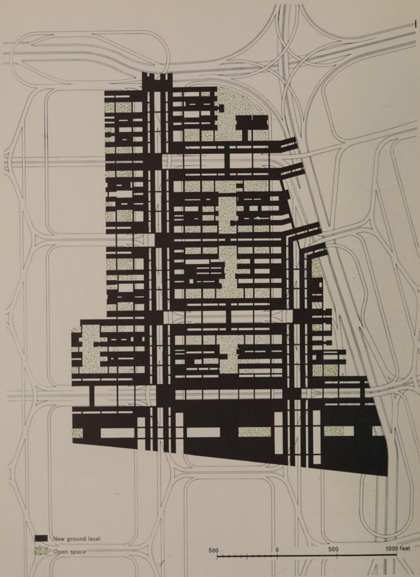
181 The design for complete redevelopment—plan at 'new ground' level showing in black the new perforated deck on which the new buildings would arise.
