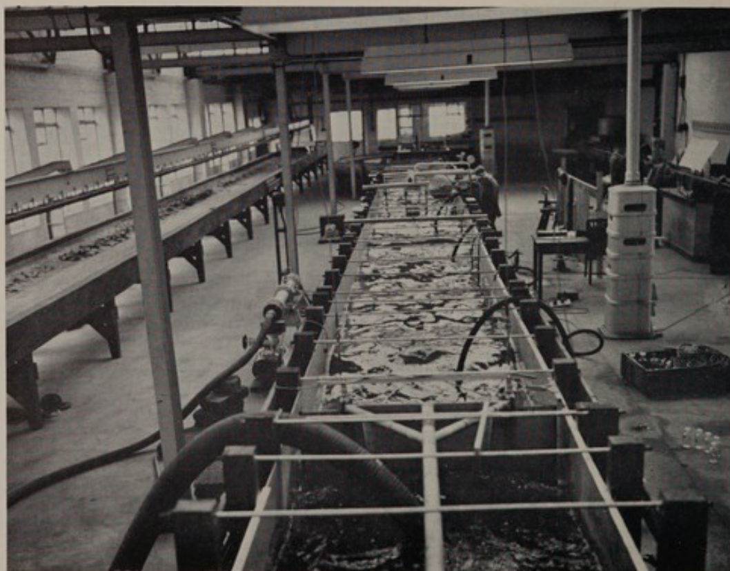
PLATE 20. Wave tank at British Transport Dock Board Research Station, used for experiments on reaeration
